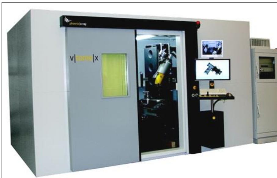
Figure D.1. The General Electric Phoenix V|Tome|X L240 X-ray \mu CT scanner used for acquiring X-ray images.
