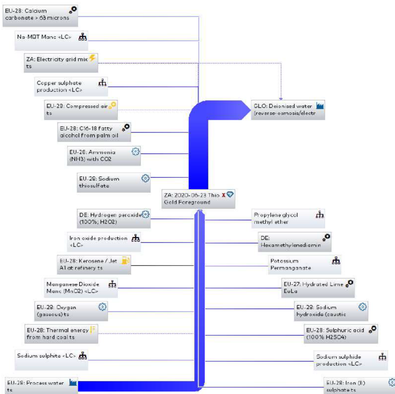
Figure 0-2: GaBi® plan for thiosulphate leaching flowsheet LCA
