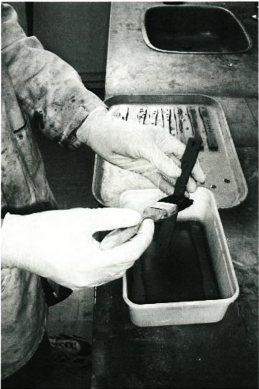
Figure 4.22: Illustration of infiltrations with epoxy resin
