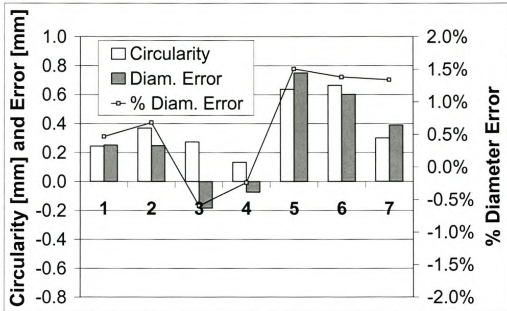
Figure 5.10: Circularity of the LOM Process.
