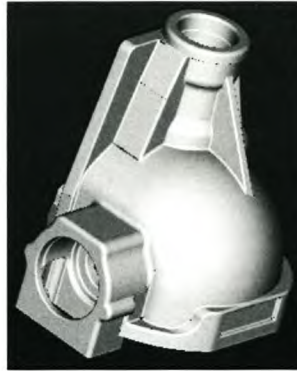
Figure 4.4: Benchmark part used for geometric accuracy
