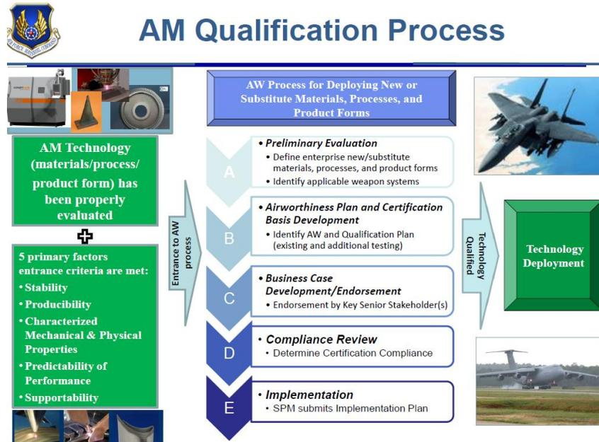
Figure 1.5: Proposed AM qualification process for aerospace (Naguy 2014)
