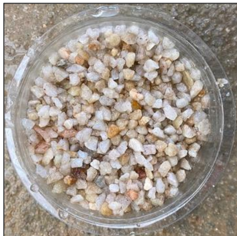
Figure F- 6: Core rocks D_{50} = 5\text{mm}
