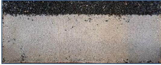
Figure L- 1: Scour image Test A1-6S
