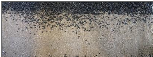
Figure L- 2: Scour image Test A1-8S
