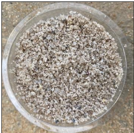
Figure F- 2: Screed layer material (grading 0.9 - 3.4mm)
