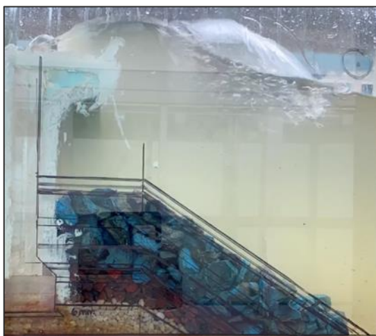
Figure 4-1: Overtopping in Test B2-16S
