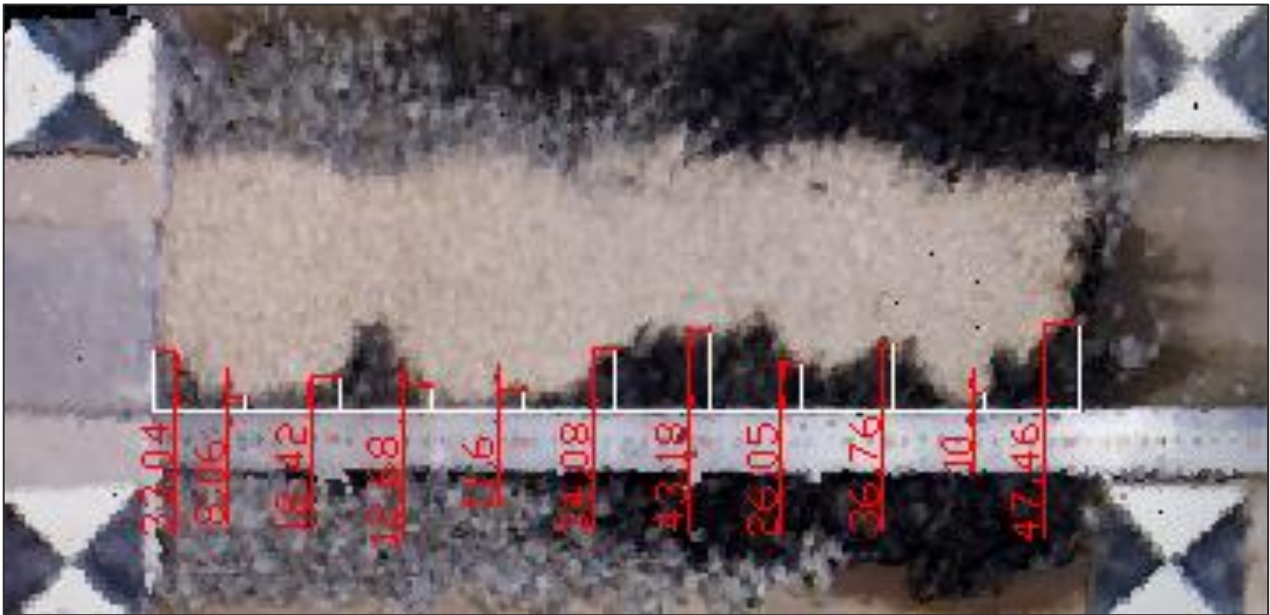
Figure I- 1: Imported scour image from the Handheld 3D scanning tablet
