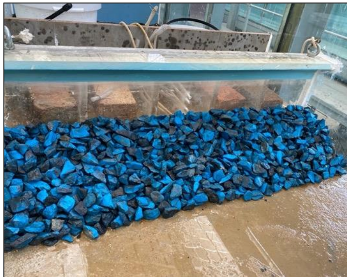
Figure H- 4: Armour layer packed over the filter layer
