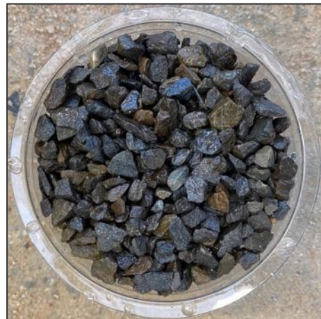
Figure F- 5: Core rocks D_{50} = 6\text{mm}
