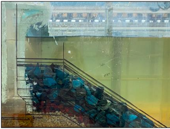
Figure 4-10: Test B3-6S before deformation of the rubble-mound structure
