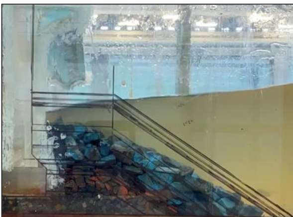
Figure 4-3: Wave drawback in Test A1-6S
