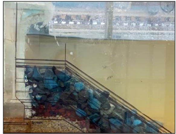
Figure 4-11: Test B3-6S after deformation of the rubble-mound structure
