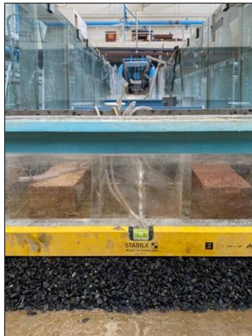
Figure H- 2: Remaining part of core packed in front of the seawall
