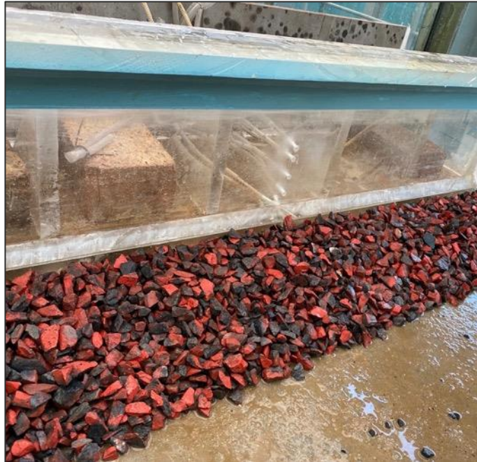
Figure H- 3: Filter layer packed over the core
