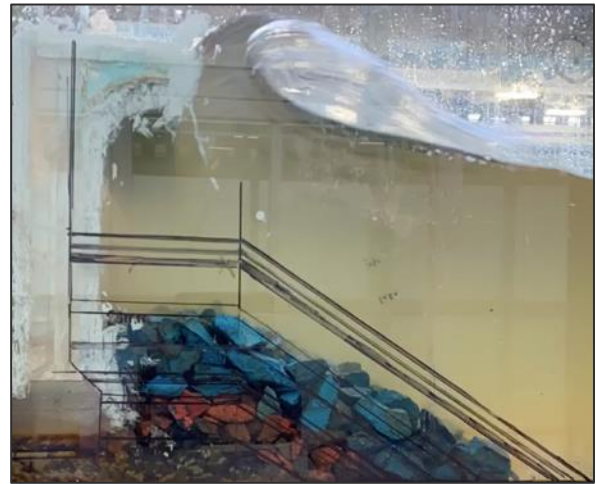
Figure 4-6: Wave breaking against the seawall in Test A1-14S
