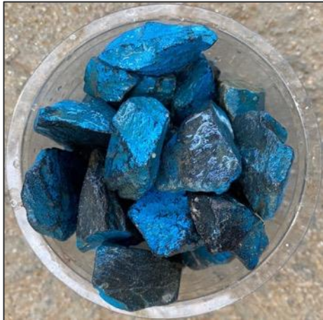
Figure F- 1: Armour layer rocks D_{50} = 28\text{mm}
