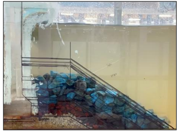
Figure 4-8: Test B3-18S after deformation of the rubble-mound structure
