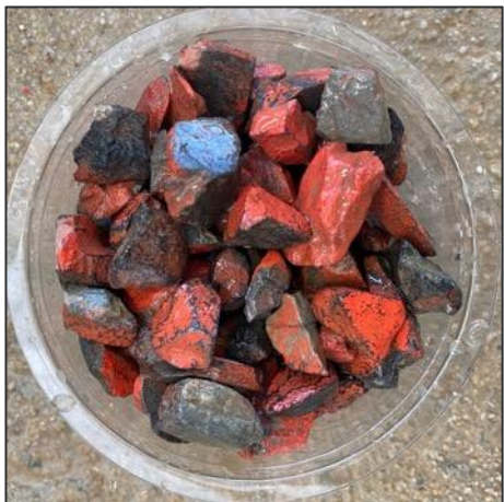
Figure F- 3: Filter layer rocks D_{50} = 13\text{mm}
