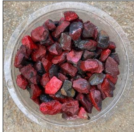
Figure F- 4: Filter layer rocks D_{50} = 11\text{mm}
