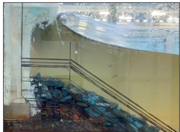
Figure 4-4: Wave breaking against the seawall in Test A1-
