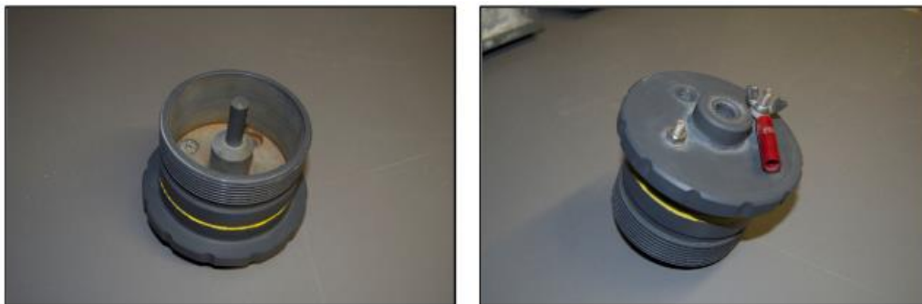
Figure 2.24 Luggin (left) and connection point (right) of chloride conductivity cell (UCT, 2017)
