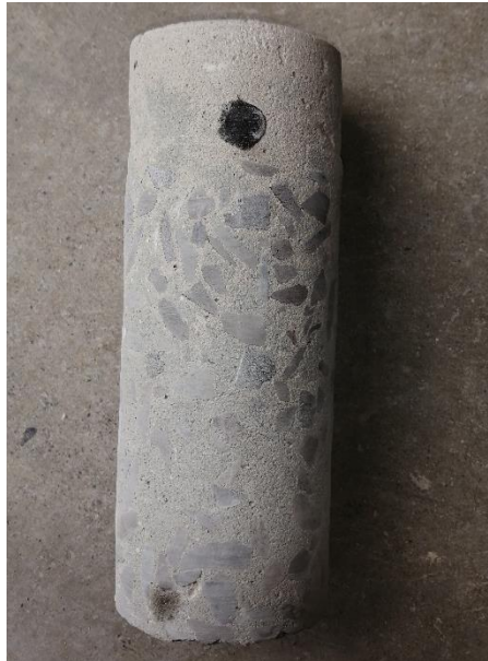
Figure 3.13 Durability core, drilled through the top of the rod
