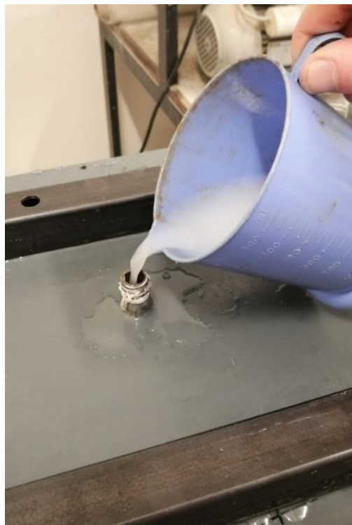
Figure 3.45 Calcium hydroxide solution added to in the chamber through the lid
