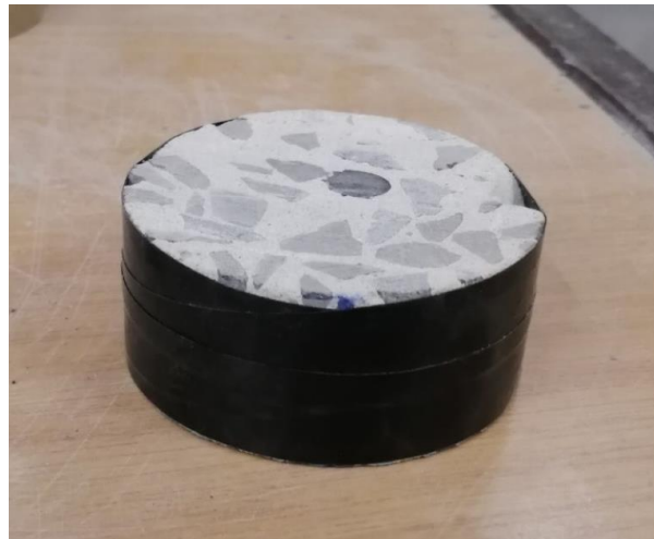
Figure 3.37 Prepared concrete specimen with packaging tape to seal the sides
