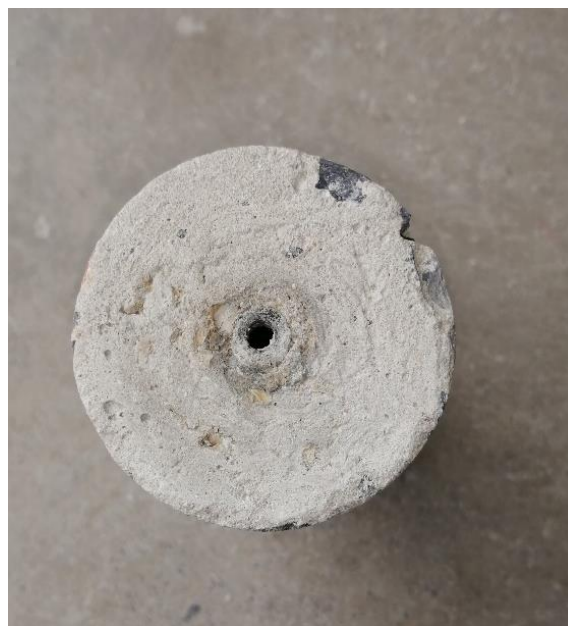
Figure 3.12 Top view of crack severity core, with the rod in the centre
