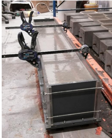
Figure 3.5 Beam after being cast, with thin layer of moisture on exposed surface
