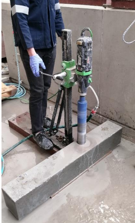
Figure 3.8 Beam being core-drilled
