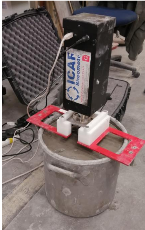
Figure 3.20 Assembled rheometer placed into concrete
