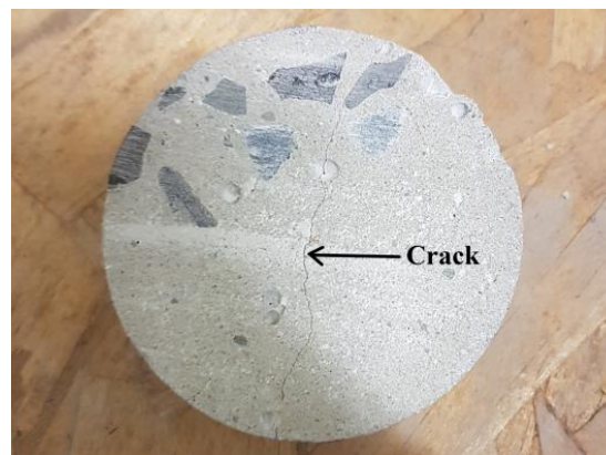
Figure 4.21 Beam 2 OPI sample top crack
