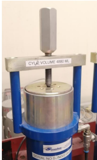
Figure 3.30 The specimen and housing placed on the permeability cell, with the coverplate tightened
