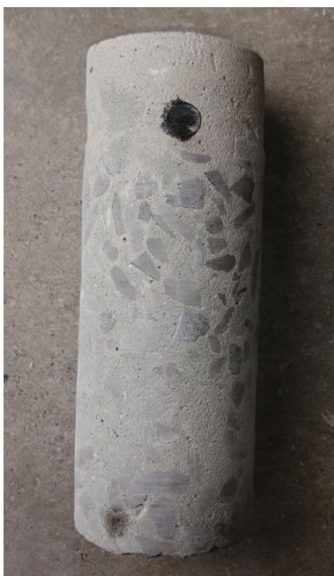
Figure 3.26 Concrete core drilled from the top
