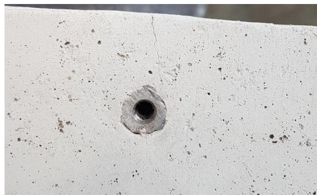
Figure 4.5 Slightly visible voids and tensile cracks at the reinforcement
