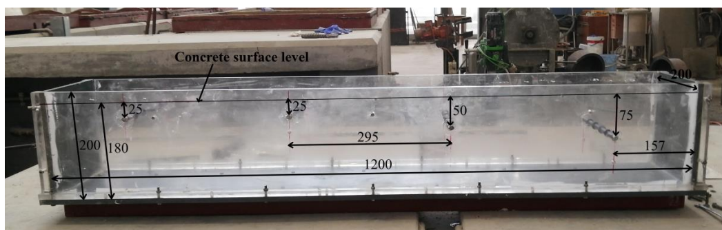
Figure 3.3 Beam mould with dimensions in mm
