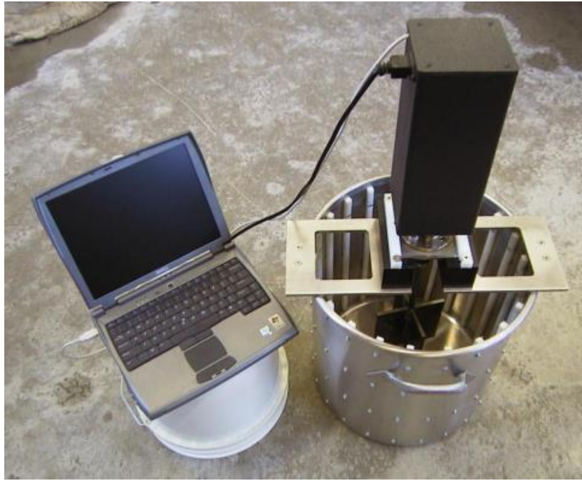
Figure 3.19 ICAR Rheometer components assembled (GI, 2016)
