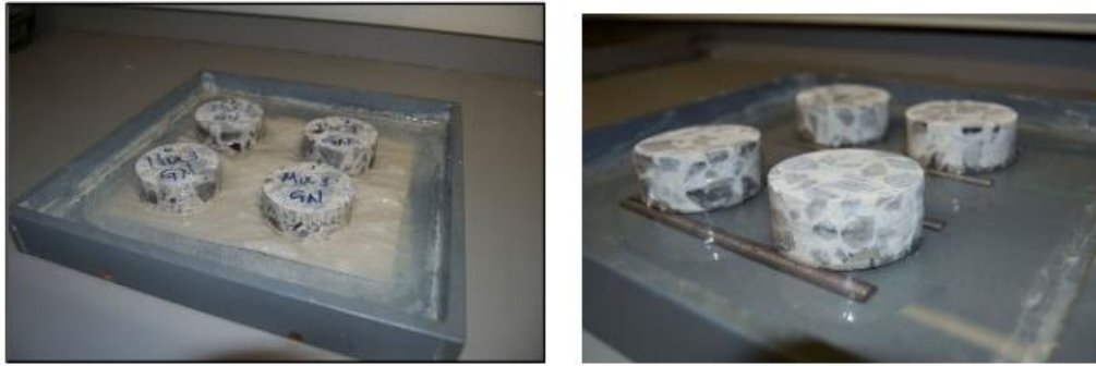
Figure 2.21 Examples of the sorptivity test being conducted (UCT, 2017)
