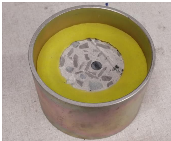
Figure 3.28 Concrete specimen inside the rubber collar, placed in the rigid sleeve
