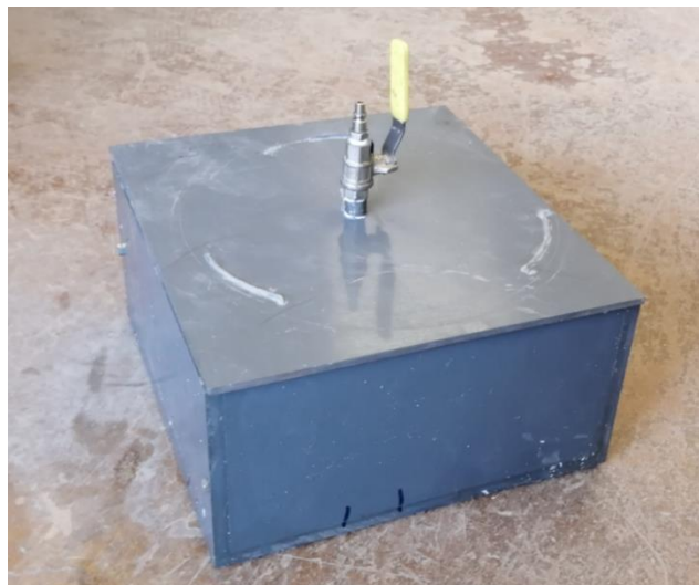
Figure 3.40 Valve inserted in the lid to connect the vacuum pump
