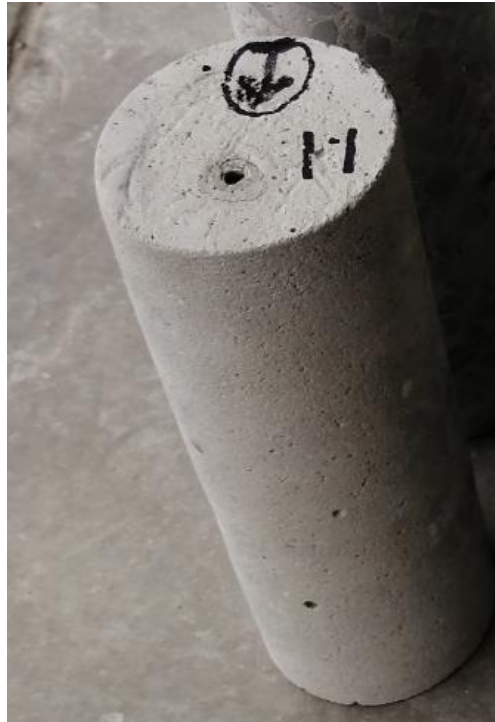
Figure 3.34 Crack severity core, drilled from the side of the beam over the reinforcing rod
