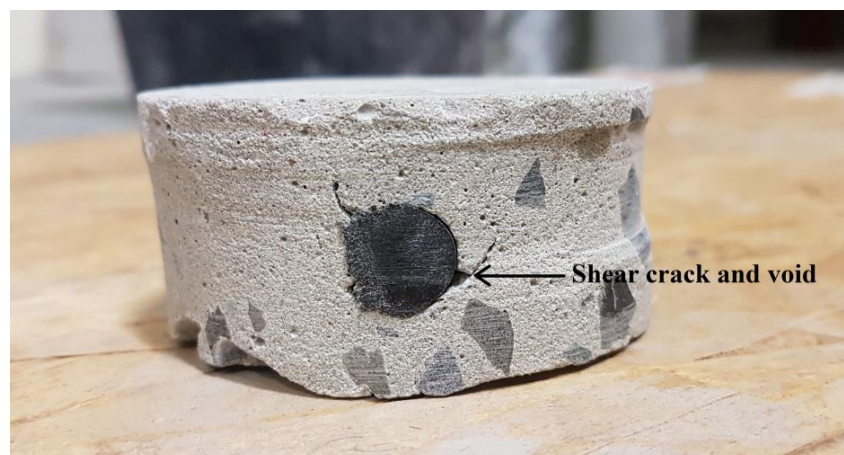
Figure 4.42 Beam 5 OPI sample front crack
