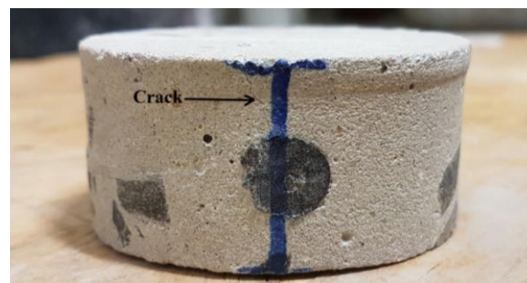
Figure 4.22 Beam 2 OPI sample front crack
