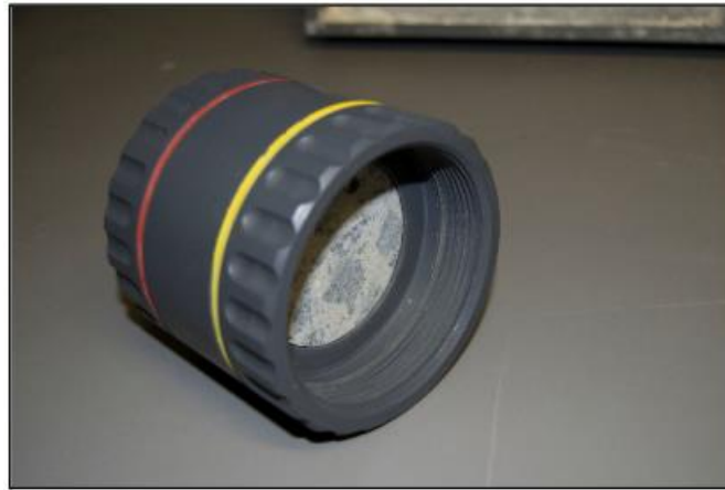
Figure 2.25 Properly placed specimen in collar (UCT, 2017)
