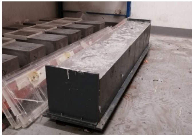
Figure 3.7 Side panels of the mould removed
