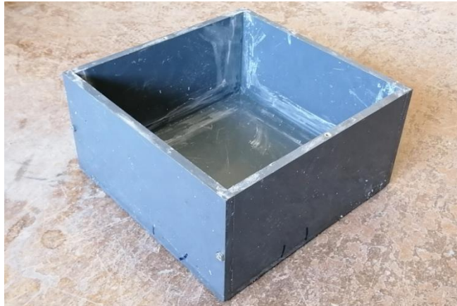
Figure 3.38 Mould used to build the vacuum saturation facility
