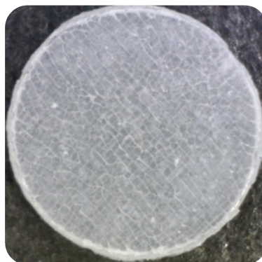
Figure 36: Photo of the surface cracks on the CPP sample subjected to 130 W/m 2 UV radiance
