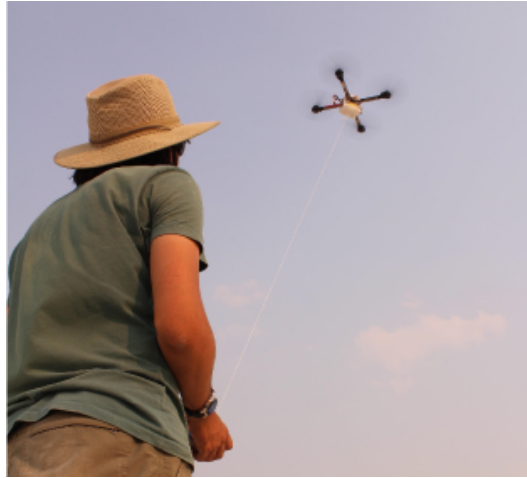
Figure 2.1: Demonstration of the Fotokite System (Lupashin and D'Andrea, 2013)
