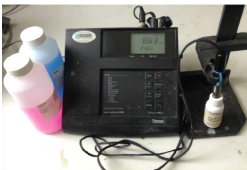
Figure 5. 5 The thermo Orion 420A+ pH meter with the two standard pH buffers besides it
