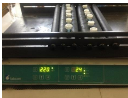
Figure 5. 6 The SPL-MP15 Alcon linear platform shaker with the instrumental parameters shown
