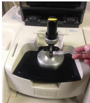
Figure 2. 3 Avatar IR (ATR) instrument with a ZnSe/Diamond crystal
