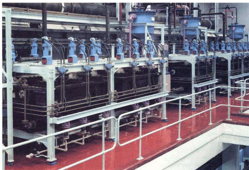
Figure 1. 4 A simple industrial design for the extraction system of platinum group metals courtesy of the Matthey Rustenburg Refiners (UK) Limited, Royston, England [23]
