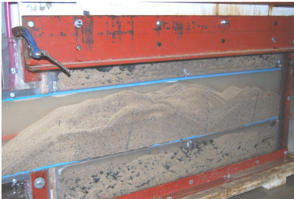
Figure 5.25: The growth of sand mounds within the Intake Pipeline
