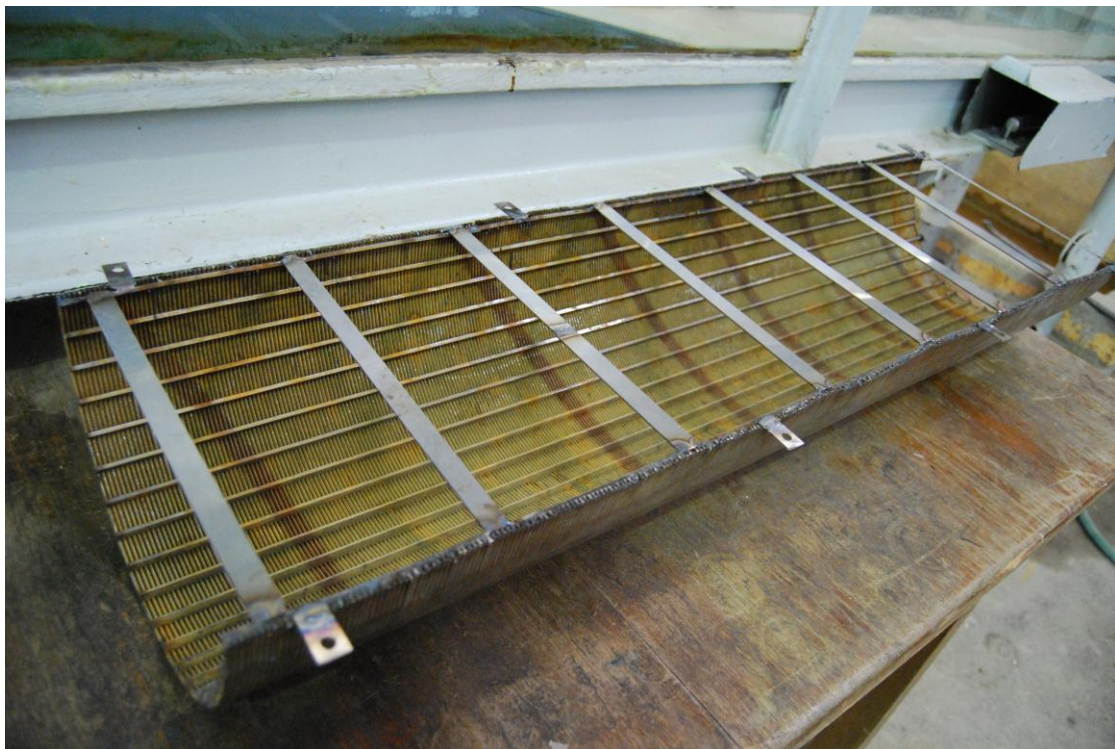
Figure 5.29: Internal View of half a \varnothing 250\text{mm} Metal Wire Pipe
