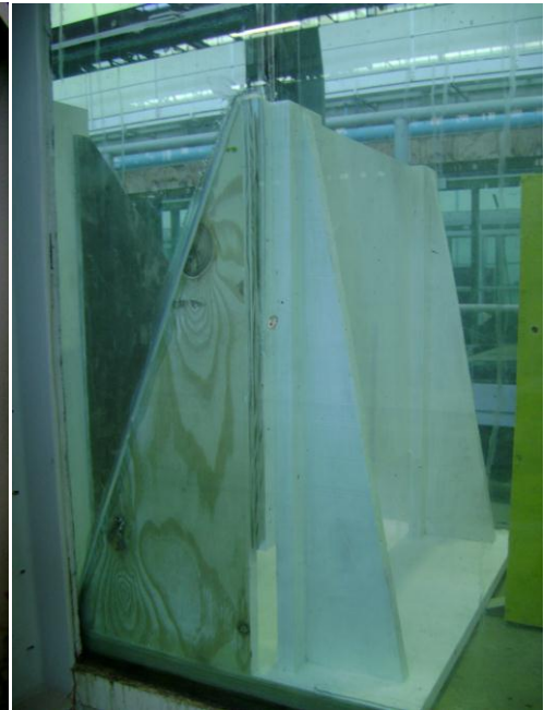
Figure B2b: Flow augmenting structure adjacent to V notch weir on the right
