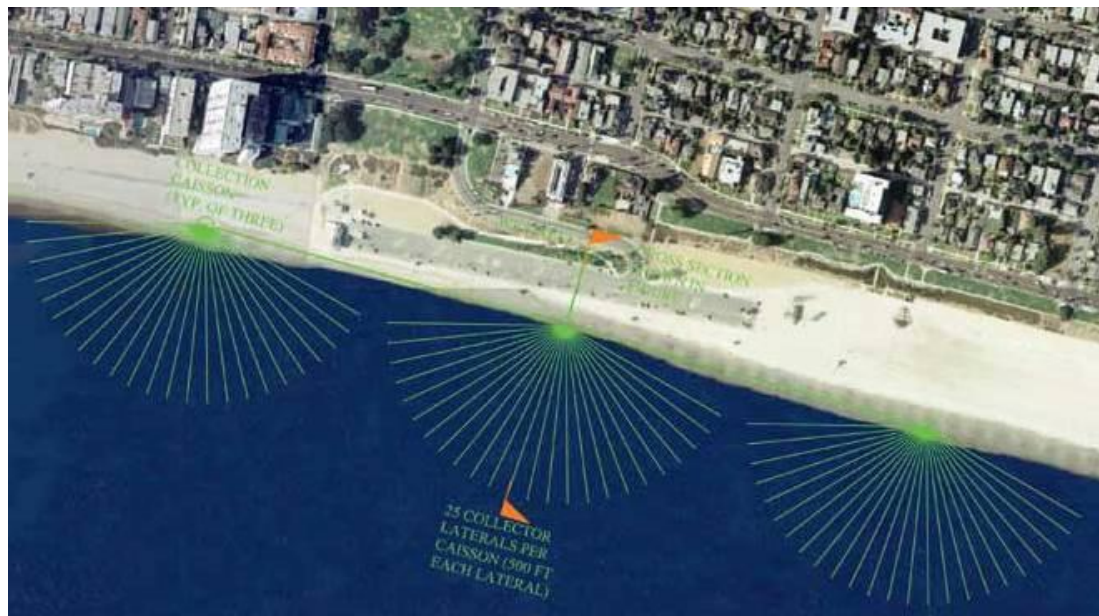
Figure 2.21: Position of radial beach wells shown on Long Beach, California (Wang, 2009)
