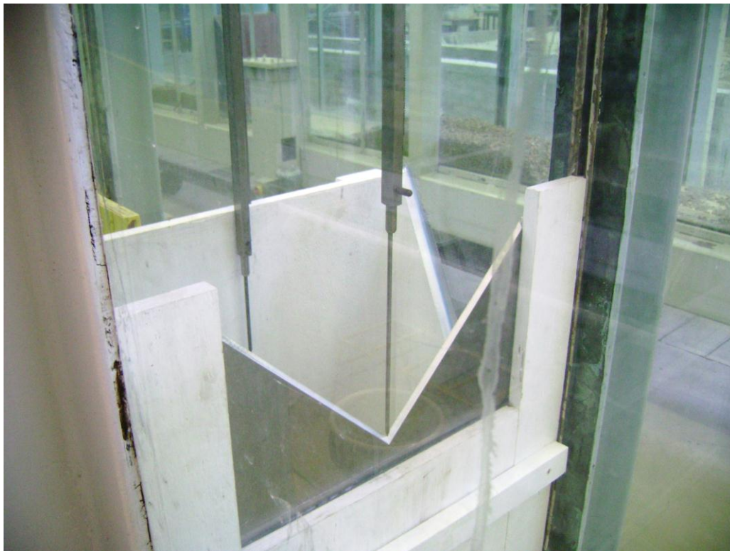
Figure B4: V notch weir with Measuring Needles
