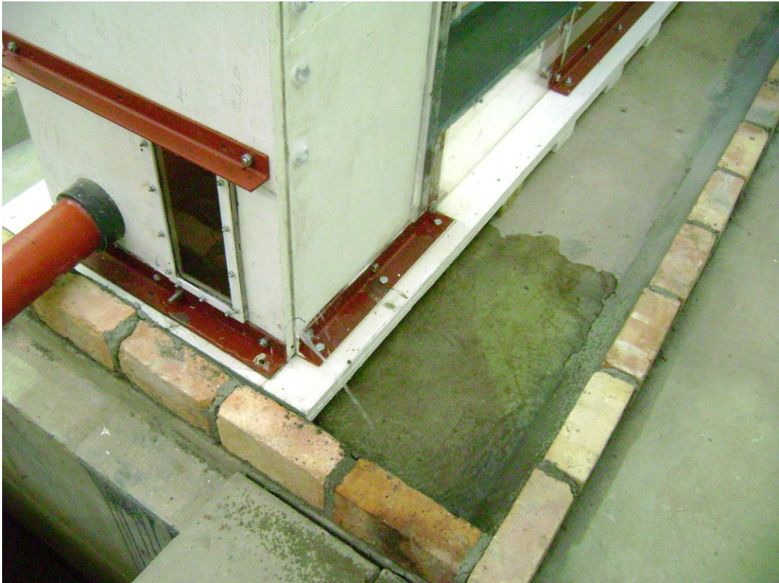
Figure 4.14: A leak in the first half of WC2 of the HPM
