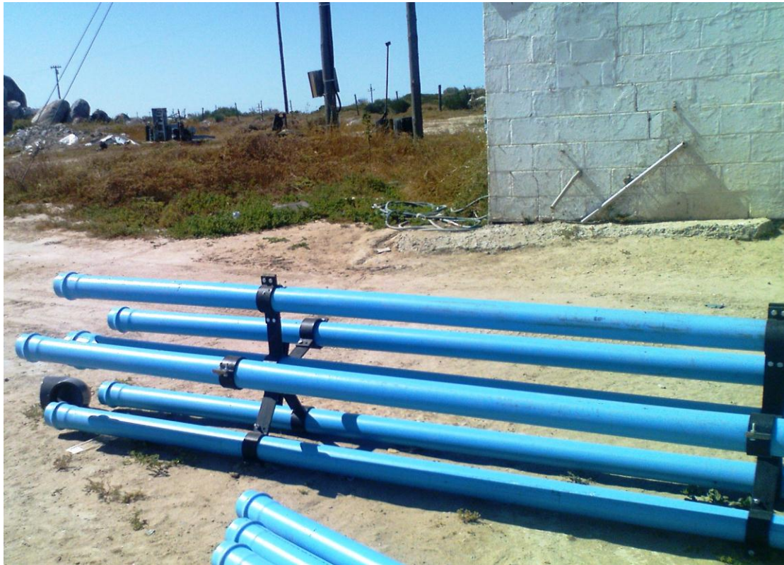
Figure 3.22: The set of pipes/jets used to displace sand
