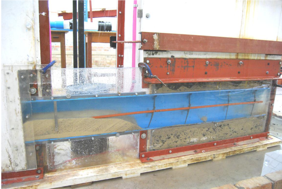
Figure 5.27: Front face of the dune has reached WC1 and the Intake pipeline has started to scour clean
