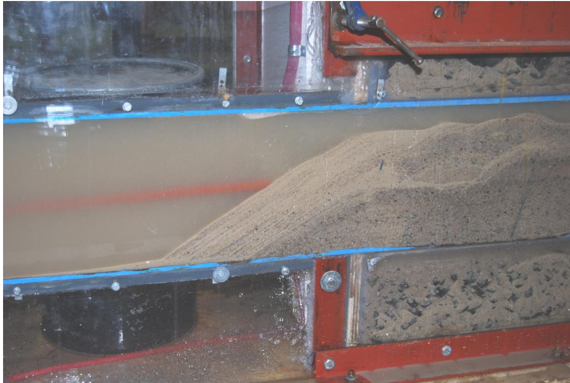
Figure 5.26: Development of front face of 'dune' seen as angular stratified layers of sand
