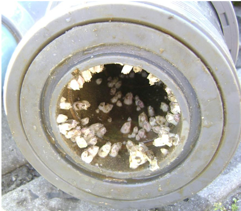
Figure 3.11: TOA - \varnothing 75mm intake pipeline and colony of Barnacles.
