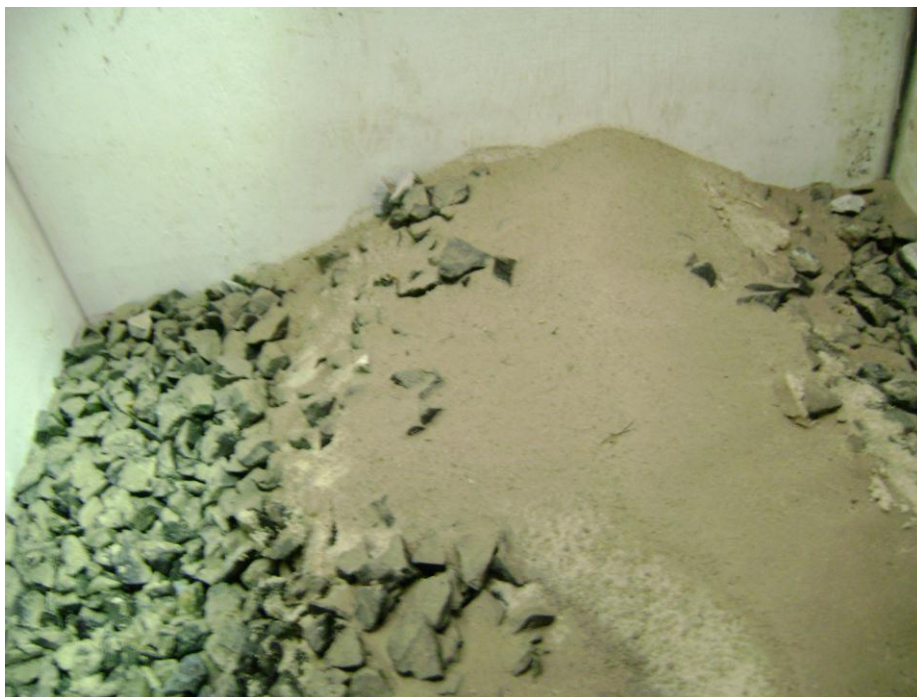
Figure 5.15: Oblique view of water column 1. Sandbar on Bedding after Back flushing with air and water. Intake pipe runs along the left edge
