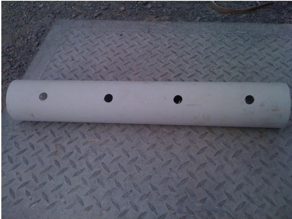
Figure 5.17: Typical Perforated PVC Pipe, similar to pipe used in Test 2
