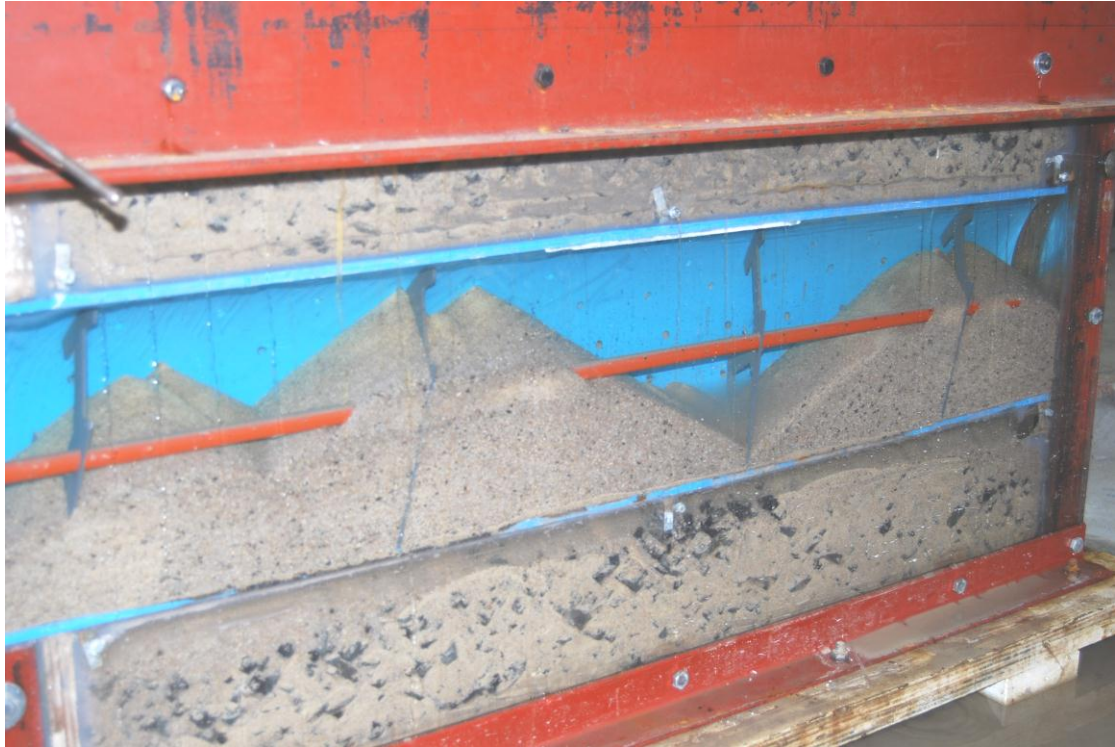
Figure 5.23: Sand ingress into Intake Pipeline before testing can commence
