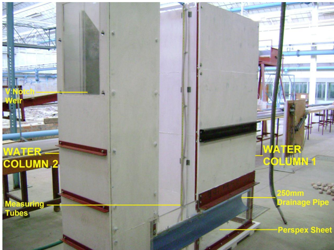
Figure 4.8: Physical Hydraulic Model for testing of Seawater Intake pipework
