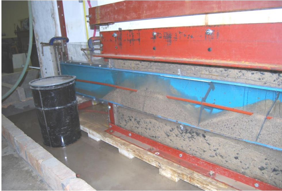
Figure 5.24: Sand ingress into Intake Pipeline when testing commences
