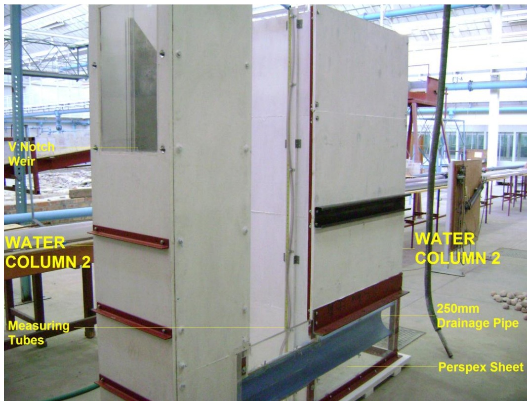
Figure A1: Hydraulic Model for testing intake pipework
