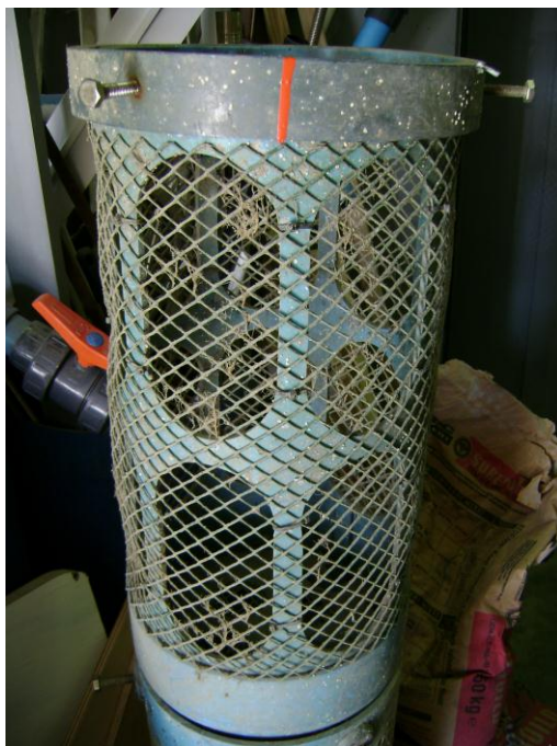
Figure 3.10: The second intake for the Two Oceans Aquarium, a \varnothing 250\text{mm} specially manufactured PVC pipe utilising Nylon mesh
