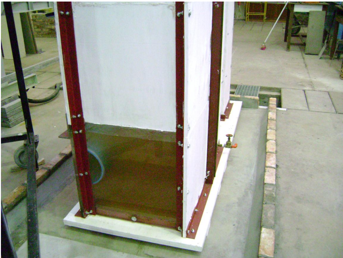
Figure 4.15: A dam constructed around the HPM
