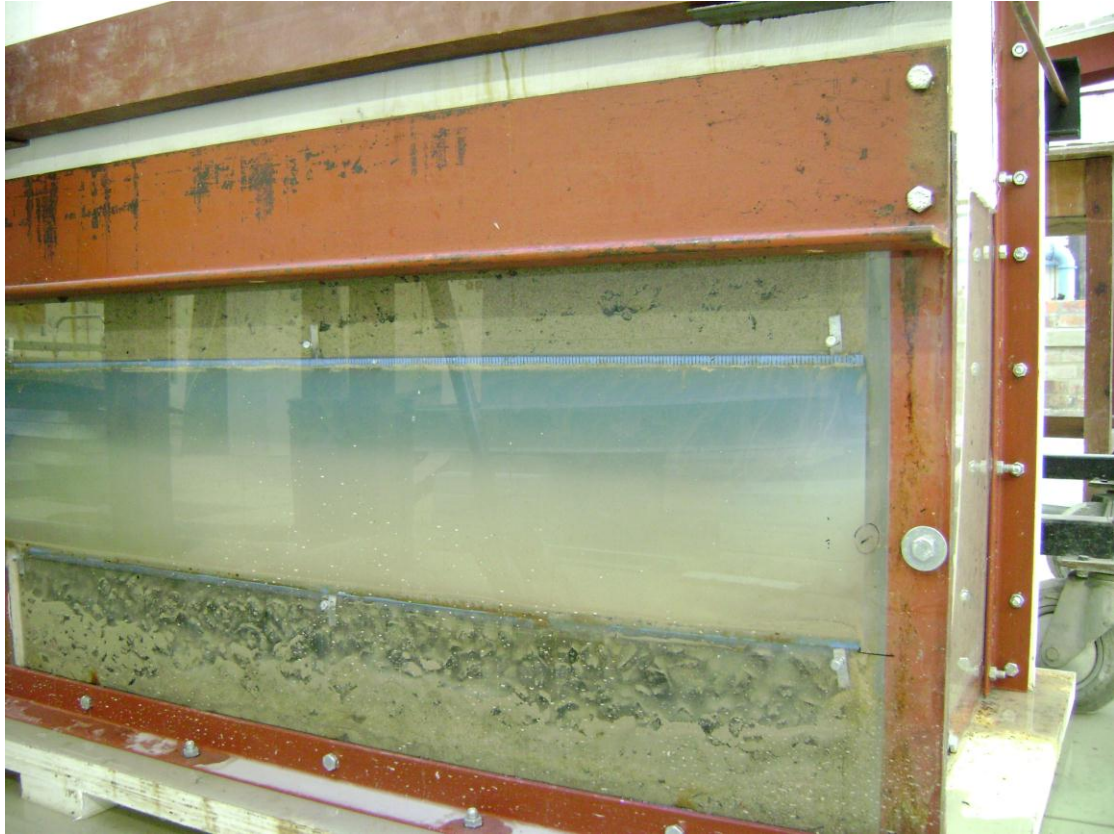
Figure 5.7: Sand and stone material surrounding the intake pipe
