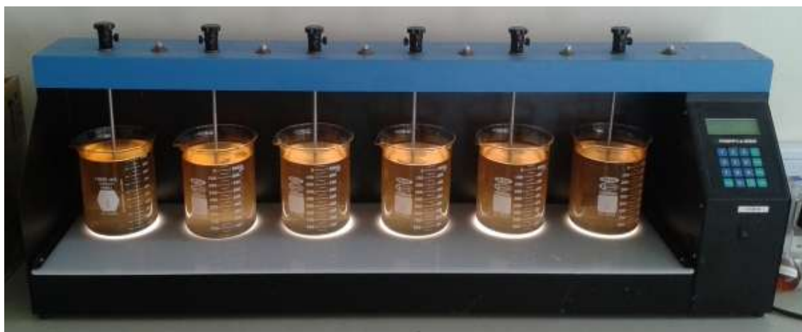
Figure 3-4: Jar test set-up during coagulation dosage determination
