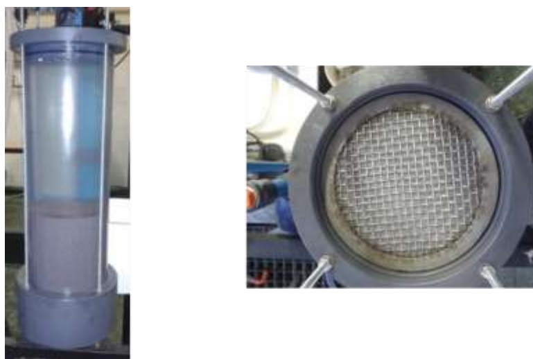
Figure 3-2: Left: PF with transparent PVC body. Right: Inside view from top showing fine sieve supported by two coarse sieves.
