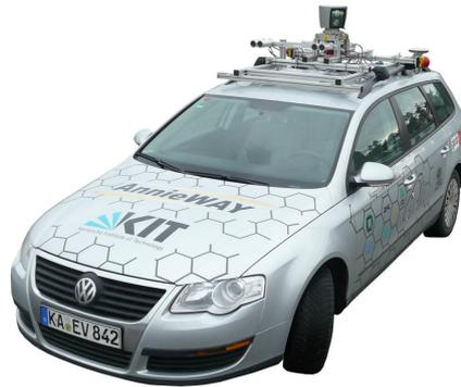
**Figure 7.11:** AnnieWay Volkswagen Passat used as a recording platform for KITTI. The recording platform is equipped with two sets of stereo cameras (colour and greyscale), a 3D Velodyne laser scanner and an inertial navigation system. Image adapted from *Vision meets Robotics: The KITTI Dataset* [123]
