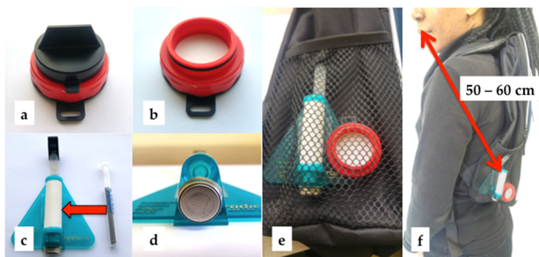
Figure A1. Photos of samplers used for personal exposure measurements: (a) Gradko rapid air NO 2 sampler (product: DIFRAM-100; UKAS method: GLM 7; detection limit: <0.2 µg/m 3 for 1-week exposure); (b) activated Gradko rapid air NO 2 sampler; (c) Radiello™ diffusive cartridge (right) and diffusive body attached to a triangular support plate (left) (products: Rad130, RAD120, and RAD121; detection limit for BTEX: 0.05, 0.01, 0.01, and 0.01 µg/m 3 , respectively; calibration: CS 2 ); (d) ACR Systems Inc. temperature logger (product: SmartButton (01-0187); detection limit: −40 °C to 85 °C); (e) air monitoring devices in the mesh pocket of a backpack (product: Barron BB0110 Curve and Arch Design backpacks); (f) backpack worn by participants with samplers located 50 to 60 cm from the face.
