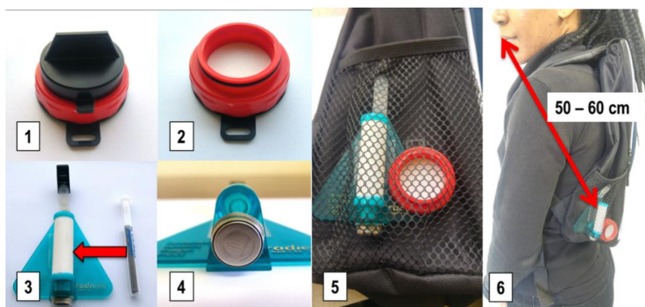
Figure 2.6. Procedures followed for personal exposure measurements. Description: 1. Gradko rapid air NO 2 sampler (product: DIFRAM-100; detection limit: <0.2 µg/m 3 for 1-week exposure). 2. Activated Gradko rapid air NO 2 sampler. 3. Radiello™ diffusive cartridge (right) and diffusive body attached to a triangular support plate (left) (products: Rad130, RAD120, and RAD121; detection limit for BTEX: 0.05, 0.01, 0.01, and 0.01 µg/m 3 , respectively; calibration: CS 2 ). 4. ACR Systems Inc. temperature logger (product: SmartButton® (01-0187); detection limit: -40 °C to 85 °C). 5. Air monitoring devices in the mesh pocket of a backpack (product: Barron BB0110 Curve and Arch Design backpacks). 6. Backpack worn by participants with samplers located 50 to 60 cm from the face. Photos taken and figure designed by the author of this dissertation based on information previously described.[521]
