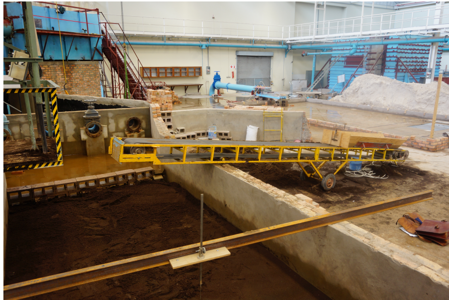
FIGURE 4.6: Sediment feed conveyor belt system
