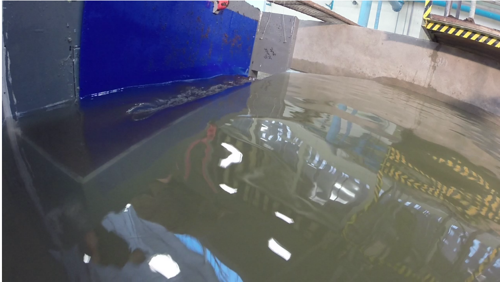
FIGURE 5.38: Flow in graveltrap of structure A, with Q_{riv} = 25.6 l/s
