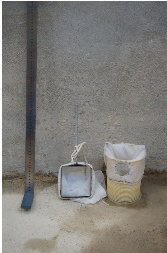
FIGURE 4.15: Survey ruler, sediment transport measuring net and the internal net of pump A (from left to right)
