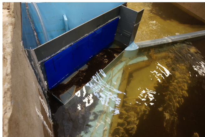
FIGURE 5.33: Sediment in the graveltrap post test SSC60
