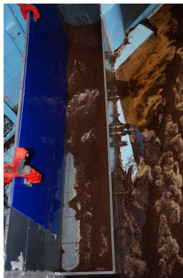
FIGURE 5.22: Sediment in the graveltrap post test SSA45
