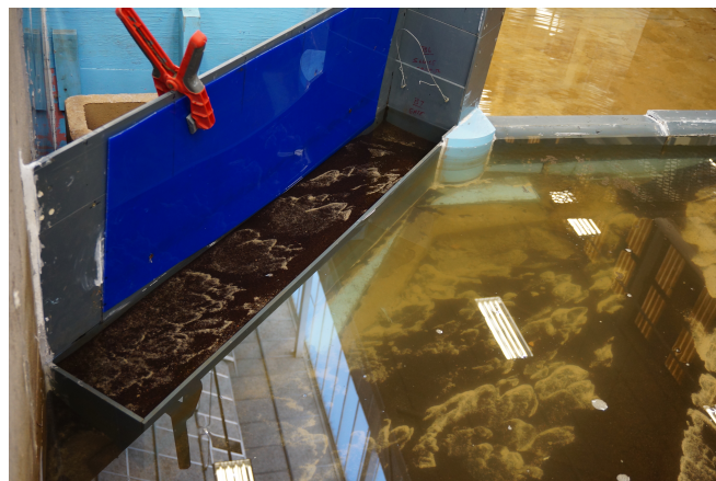
FIGURE 5.28: Sediment in the graveltrap post test SSB45
