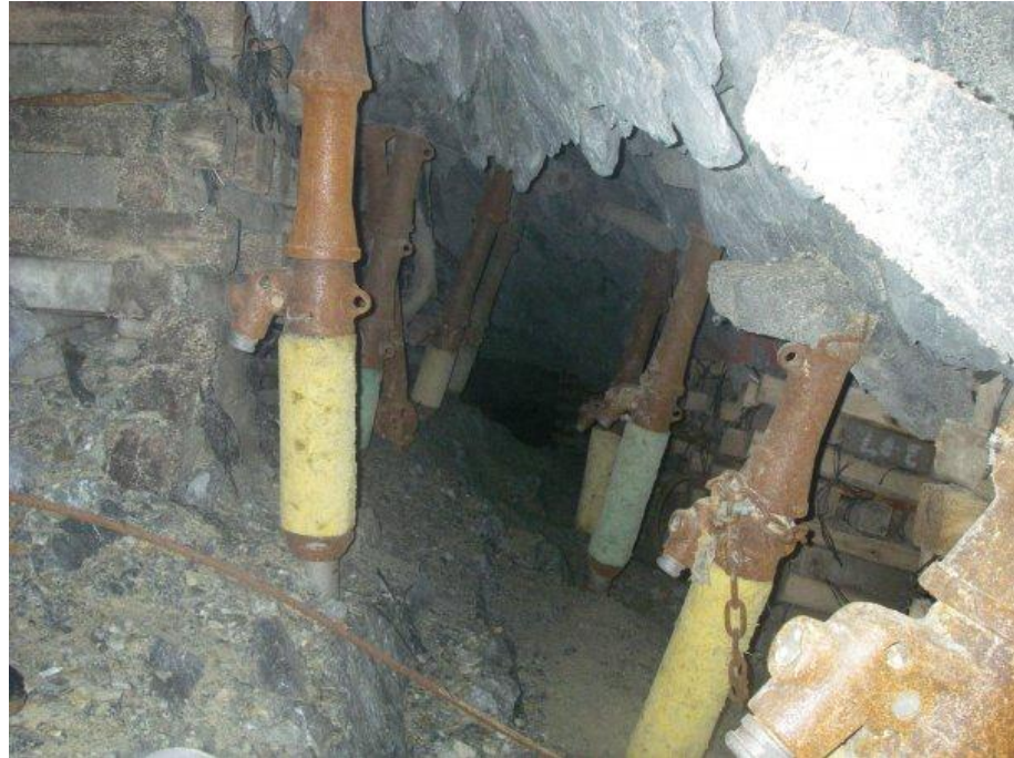
Figure 2.21: Rockprops installed at 3 shaft at Goldfields, Kloof Mine (S. Surujbally, 2007).
