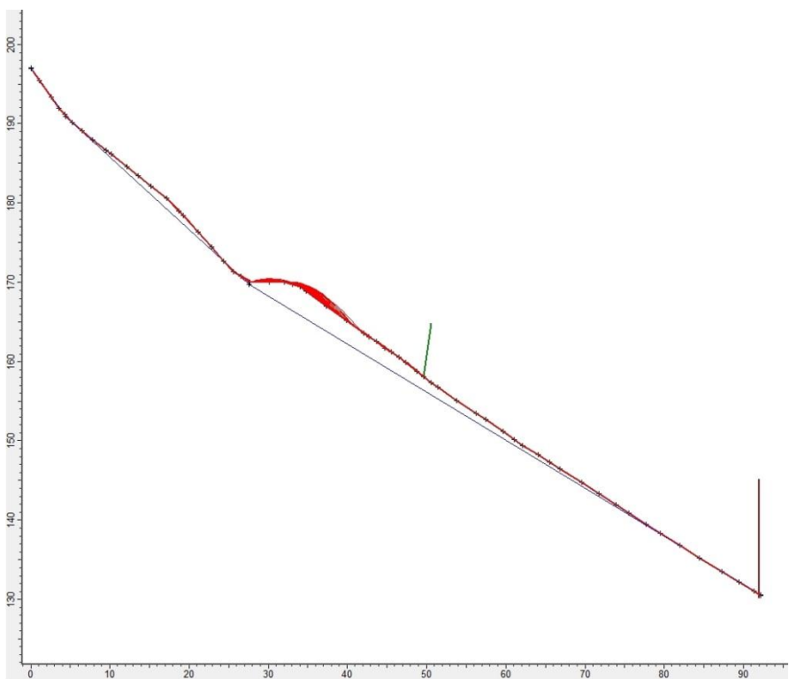
FIGURE 1.8: Rockfall simulation trajectories along 15A
