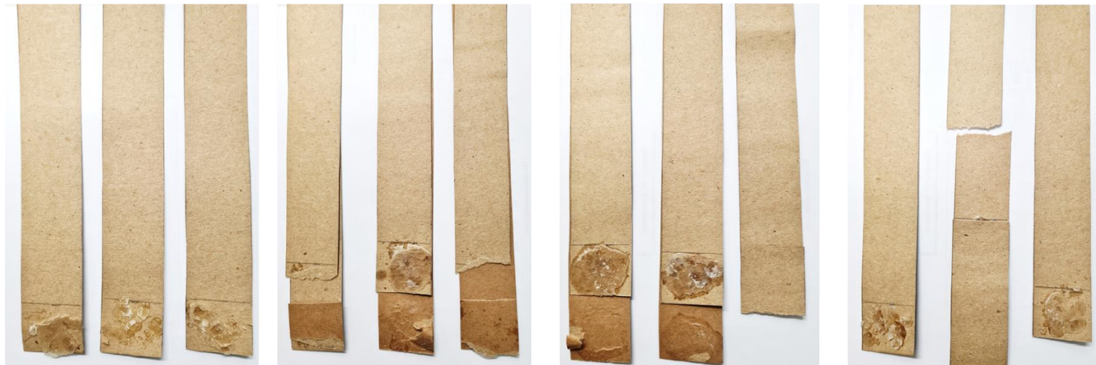
Figure 4. 17: Images of bond failure mechanisms of HEPC 30% wax HMA tensile samples
