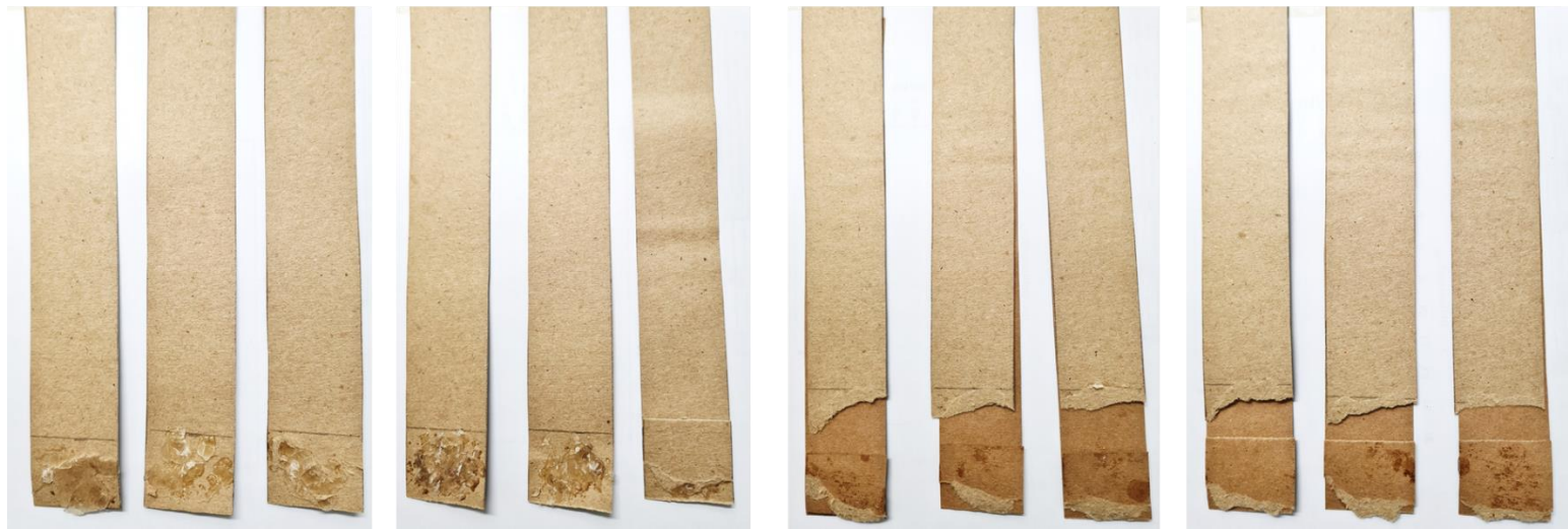
Figure 4. 16: Images of bond failure mechanisms of HEPC 10% wax HMA tensile samples
