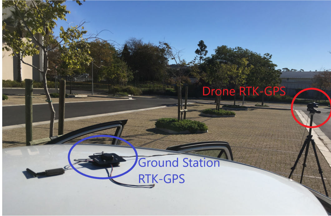
Figure 3.6: Setup of real-time RTK-GPS 33°55'38" S 18°51'55" E at 3:00 PM on the 30th of April 2018
