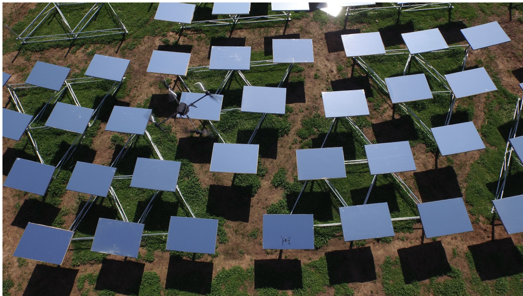
Figure 3.1: Example of a photo taken by a drone of a small-scale concentrating solar power plant viewed from the top looking down on the heliostats that are reflecting the sky. Take note of the big drone in the image and the smaller drone in the reflection of one of the heliostats. Courtesy: The TIA Helio100 project.
