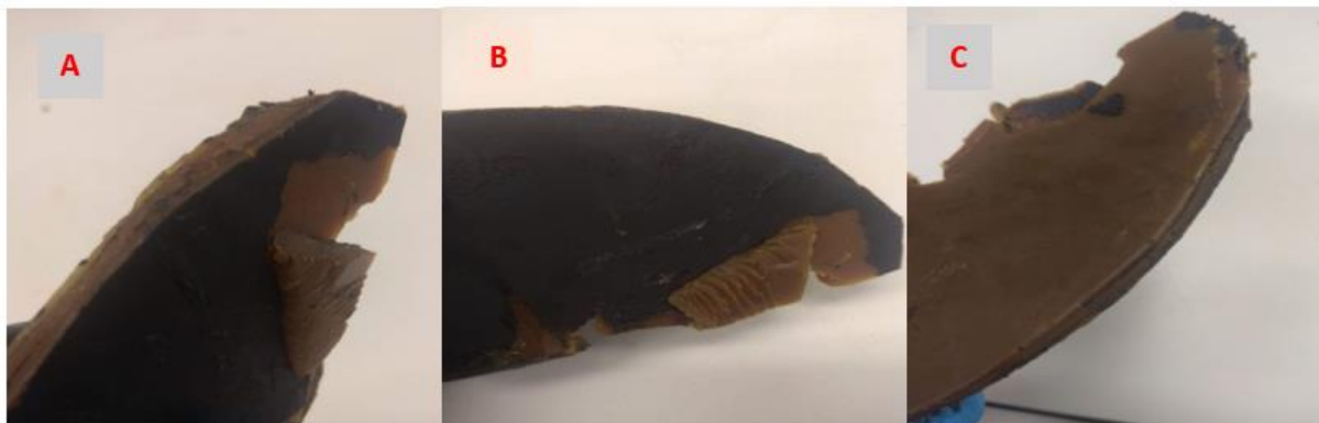
Figure 4.10. Sample of product recovered from char collection box showing layers of char (in black) and wax (in gold). (A) View showing both layers of char and wax, (B) View showing mainly char, (C) view showing mainly wax
