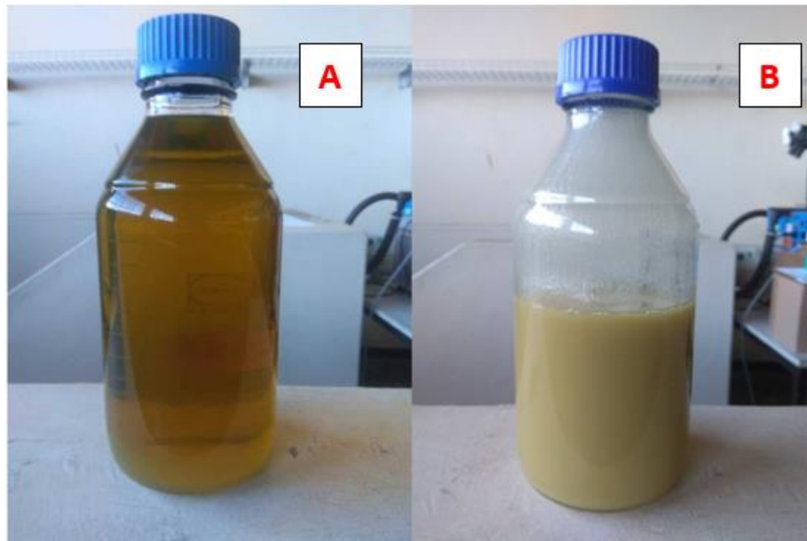
Figure 4.11. Oil samples obtained in condenser 1 at 460 °C. (A) Top light fraction, (B) Bottom waxy fraction. Samples physical appearances are similar to those recovered at 450 °C.
