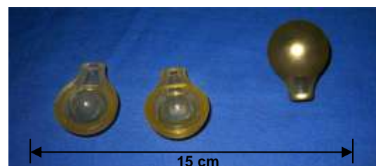
Figure 6: Prototypes of internal magnet housing
