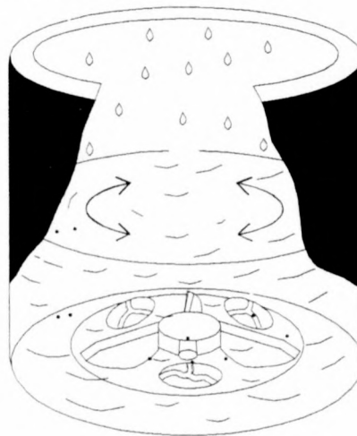
FIGURE 1.1: ILLUSTRATION OF THE BASIC MECHANICAL WASH ACTIONS OF THE THREE CATEGORIES OF WASHING MACHINES
