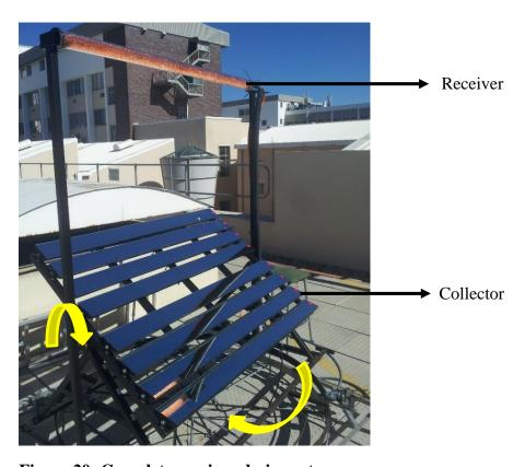
Figure 20: Complete receiver design setup
