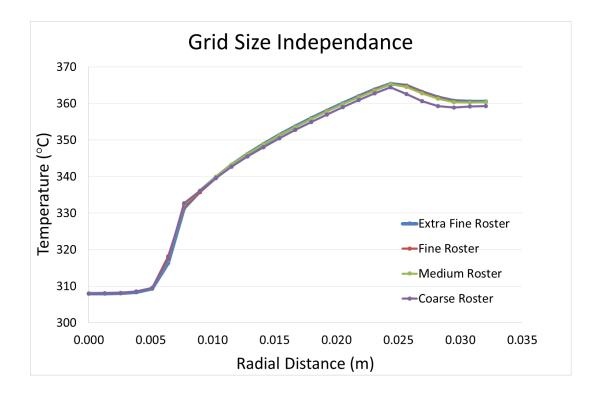
Figure 48: Verification of different mesh types in simulated model
