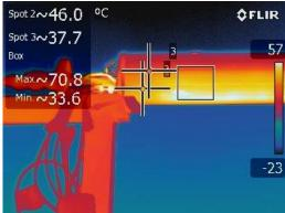
Figure 32: Thermal imaging of the receiver
