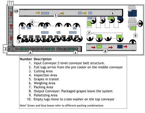
Figure 1: Facility Layout of conventional production line
