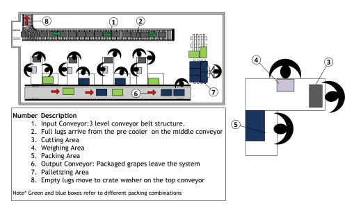
Figure 2: Facility Layout of sample production line
