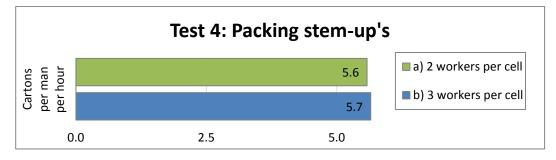
Figure 6: Summary productivity measurements of Test 4
