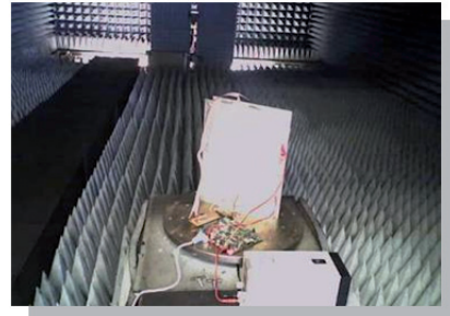
Fig. 15. Antenna rotated to -30° in anechoic chamber and beam also rotated to -30°.
