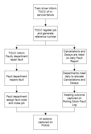
Figure 4 : In-Service Failure Process Flow
