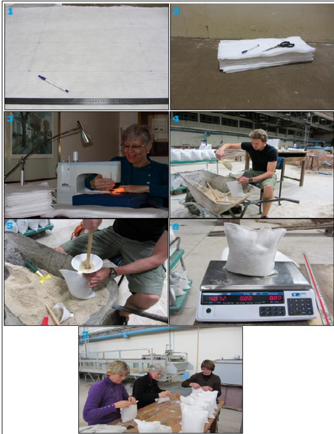
Figure 3-7: Photographs Showing the Fabrication Process of GSCs
