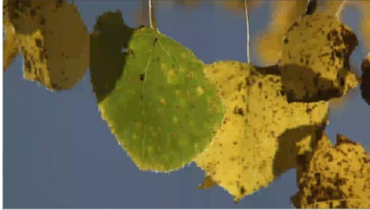
(a) Example of a video frame compressed using H.264 compression at a bit rate of 0.5 Mbit/s. Blocking artefacts are seen and motion is not smooth when the video is viewed.
