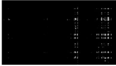
(c) Differences between a watermarked and unwatermarked frame for the SVD technique.
