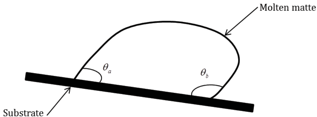
Figure 18: Effect of a tilted substrate (adapted from Eustathopoulos et al., 1999)
