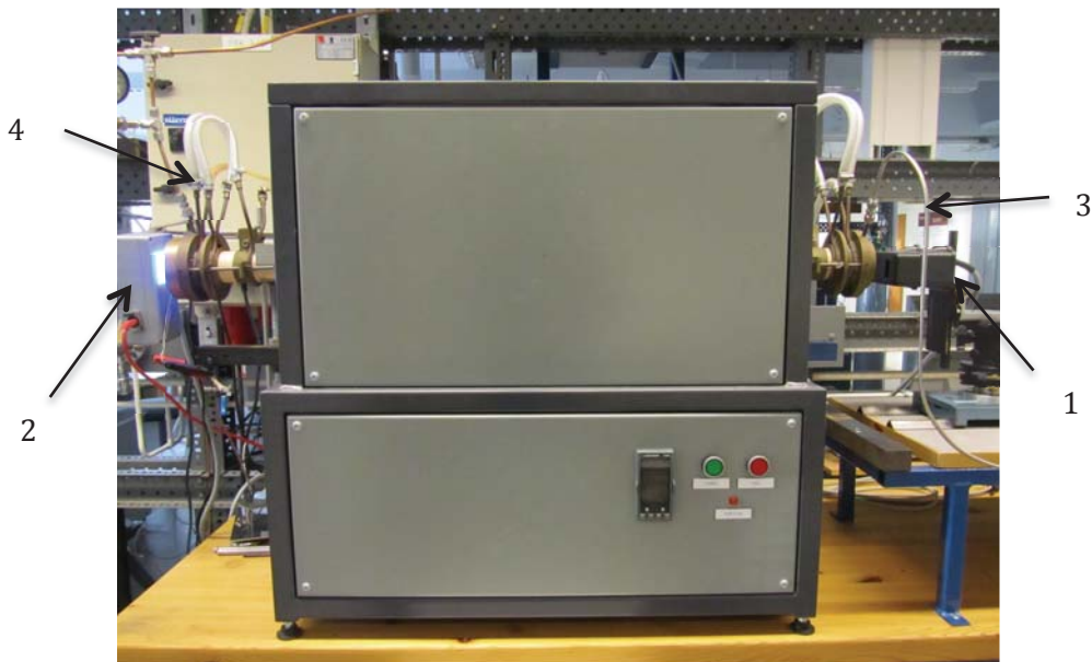
Figure 22: ENTECH, ETF 50 – 70/15 – S horizontal tube furnace (side view), Showing CMOS –HD camera (1), LED (2), and gas (3) and cooling lines (4) on both ends
