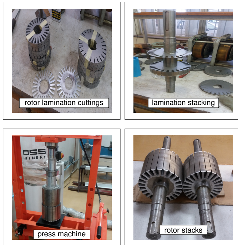
Figure 6.3: WRS and WRIM rotor lamination stacking.
