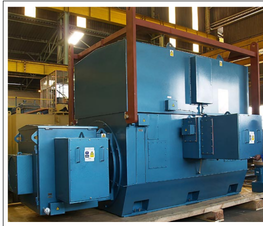
Figure 7.1: ACTOM South Africa 7 MW slip-ring mill motor [4].
