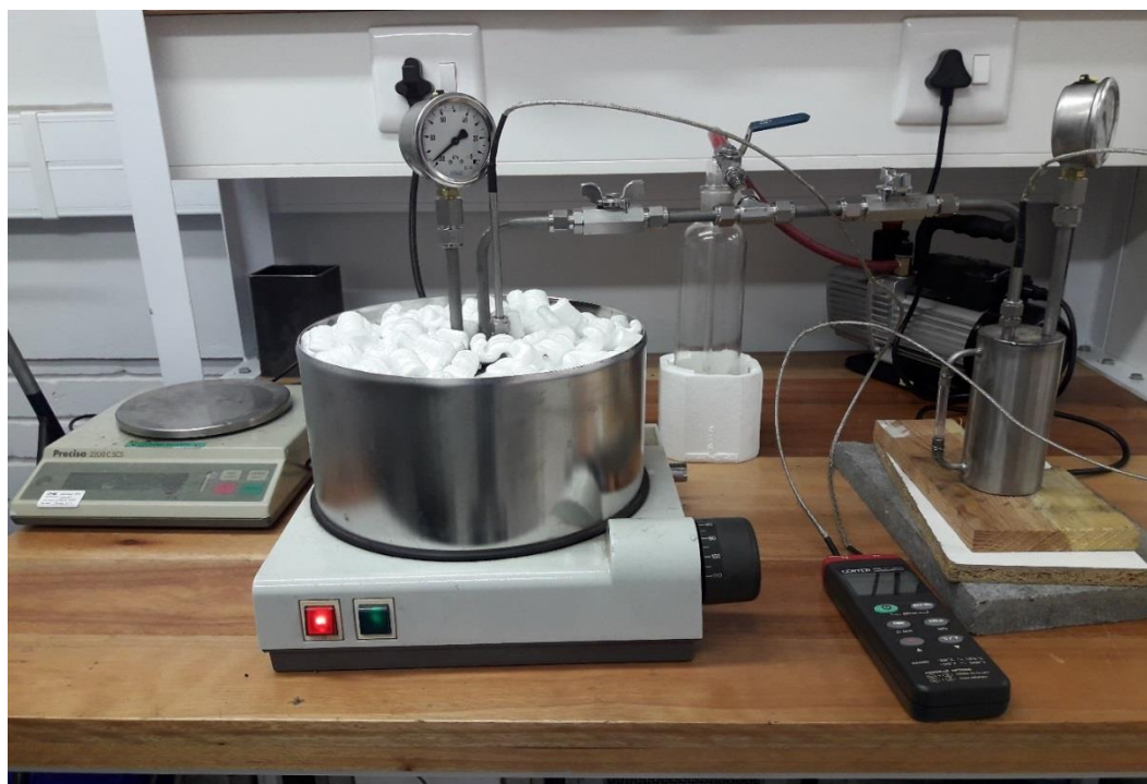
Figure 6.2 Experimental rig to study adsorption capacity of different adsorbent refrigerant pairs
