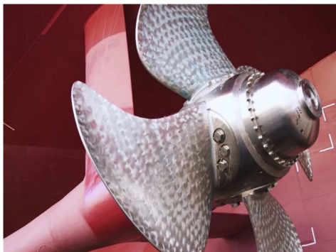
Fig. 4. The four-bladed, variable-pitch propeller of the SAA II.
