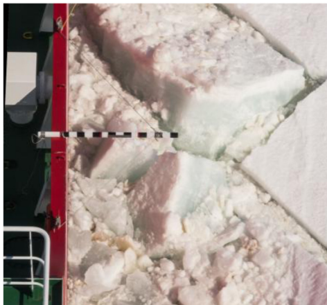
Fig. 5. The measurement stick for ice thickness estimation. Each marker is 10 cm wide.
