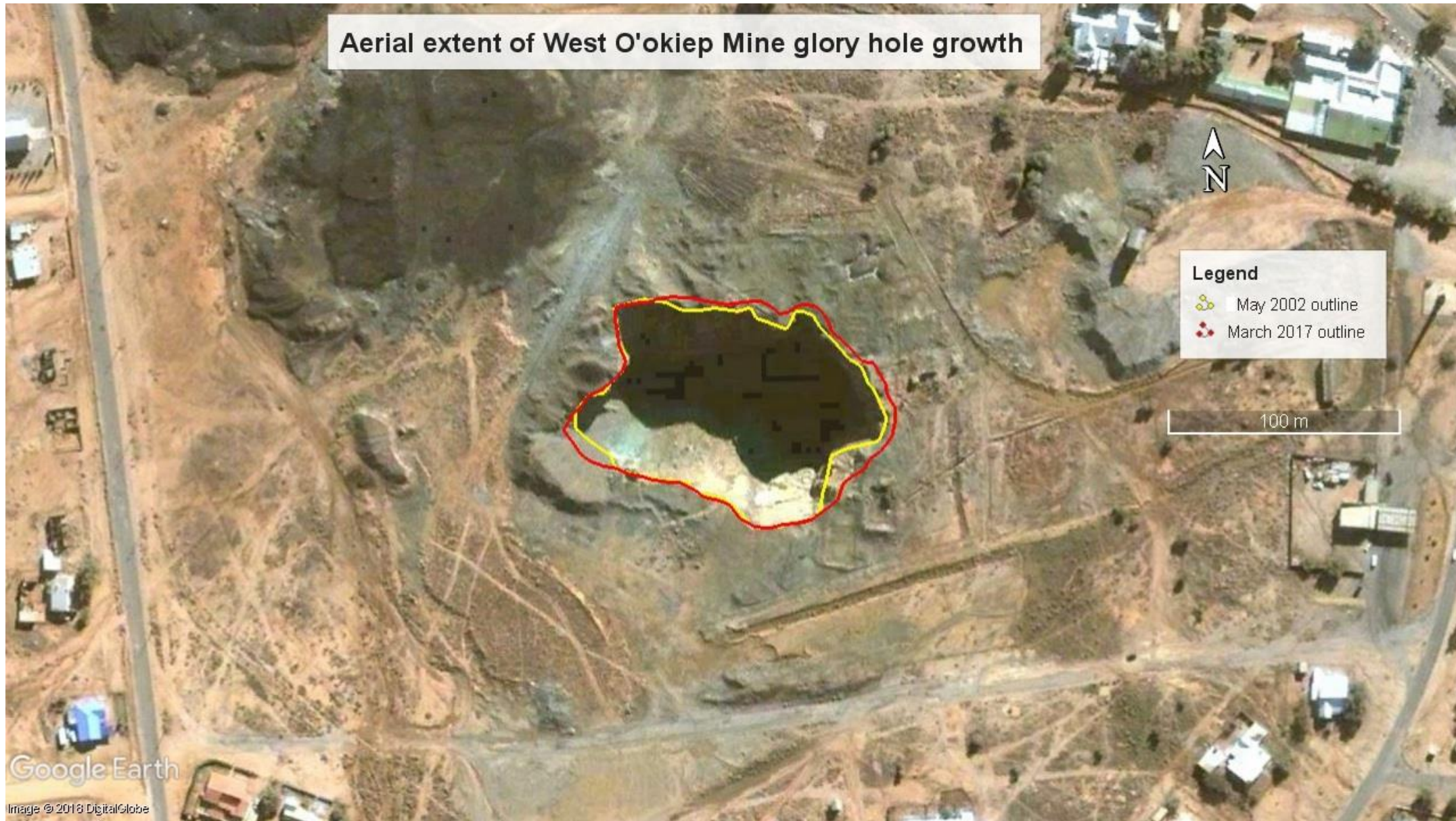
Figure 4. 7: An aerial view of the West O'okiep Mine glory hole and the extent of its growth from 2002-2017 (modified from Google Earth Pro. (2018c)).
