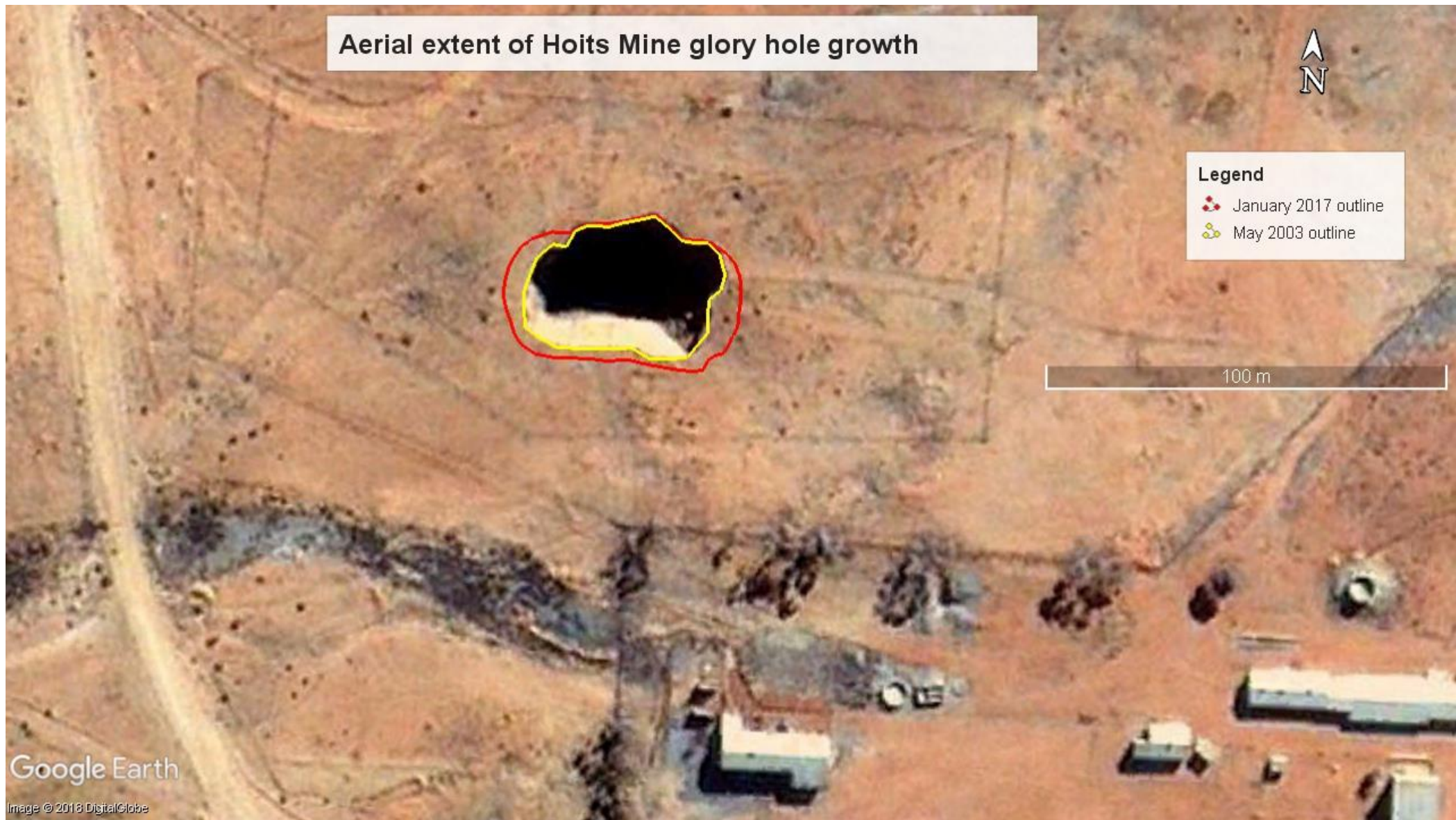
Figure 4. 12: An aerial view of the Hoits Mine glory hole and the extent of its growth from 2002-2017 (Google Earth, 2018).
