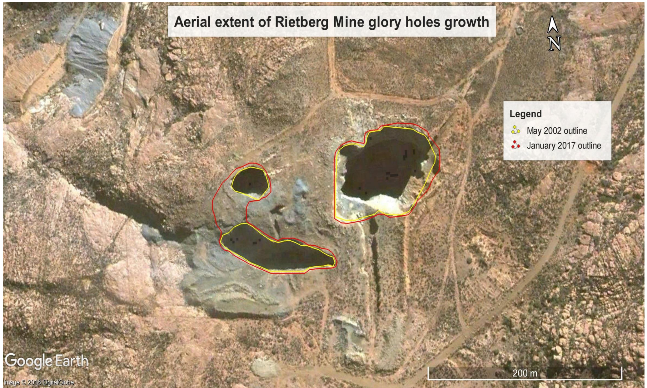
Figure 4. 3: An aerial view of the Rietberg Mine glory holes showing the extent of their growth from 2002-2017 (modified from Google Earth Pro., (2018b)).
