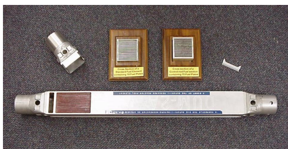
(a) A sample of a standard fuel assembly for SAFARI-1 [146]
