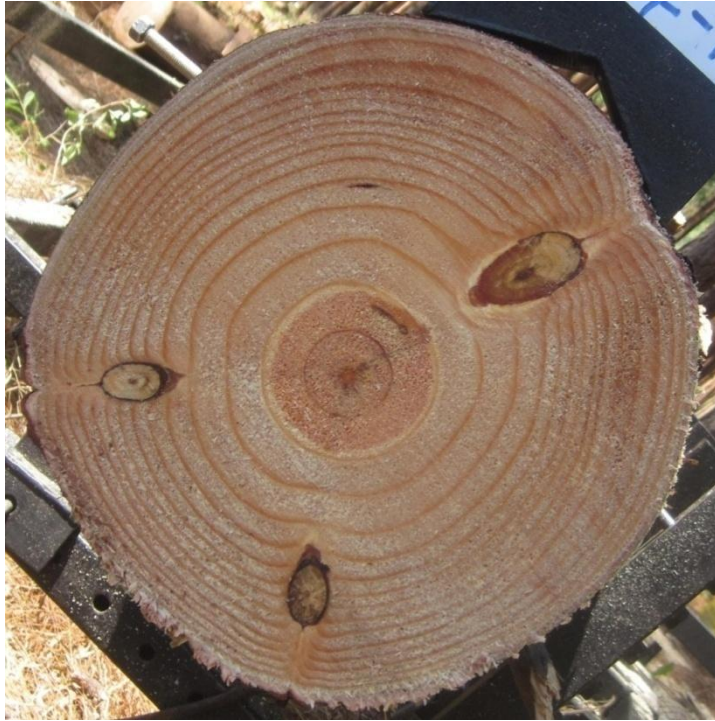
Figure 43: Resin pocket identified from photos.
