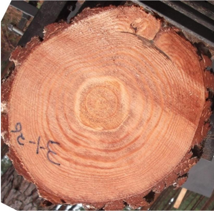
Figure 1: Resin pocket identified infield.
