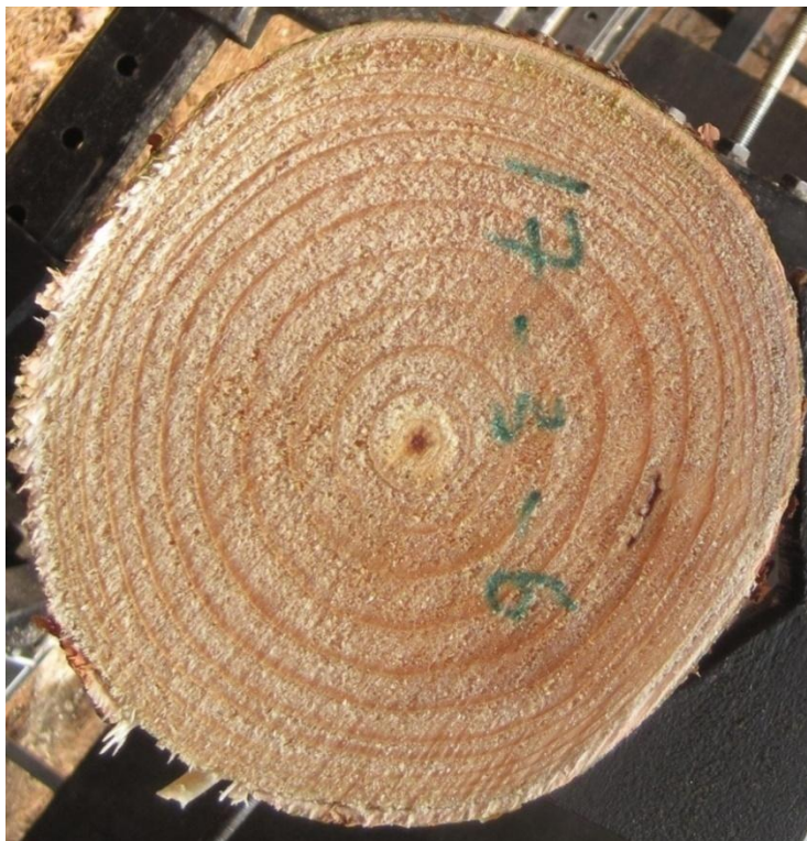
Figure 24: Resin pocket identified infield.
