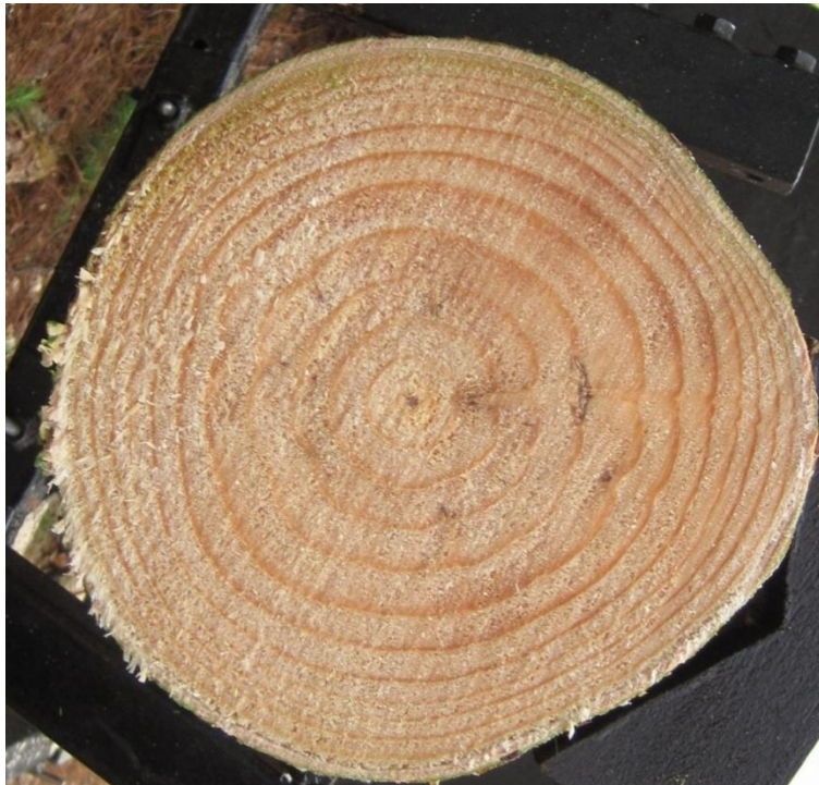
Figure 52: Resin pocket identified from photos.
