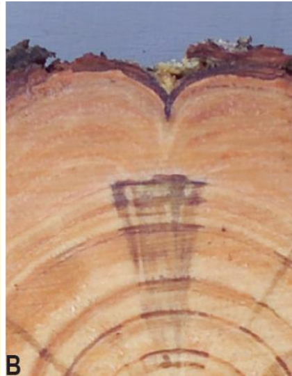
Figure 5: Type 2 resin pocket (Watt et al, 2011).
