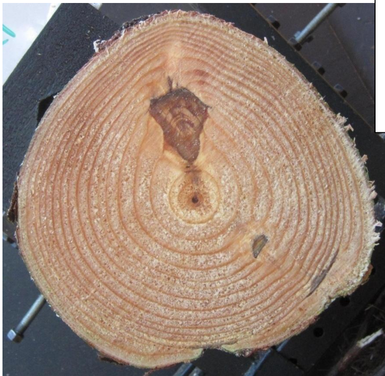
Figure 50: Resin pocket identified from photos.
