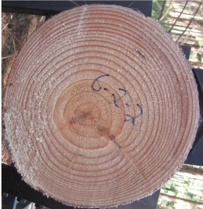
Figure 5: Resin pocket identified infield.
