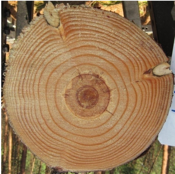
Figure 27: Resin pocket identified from photos.
