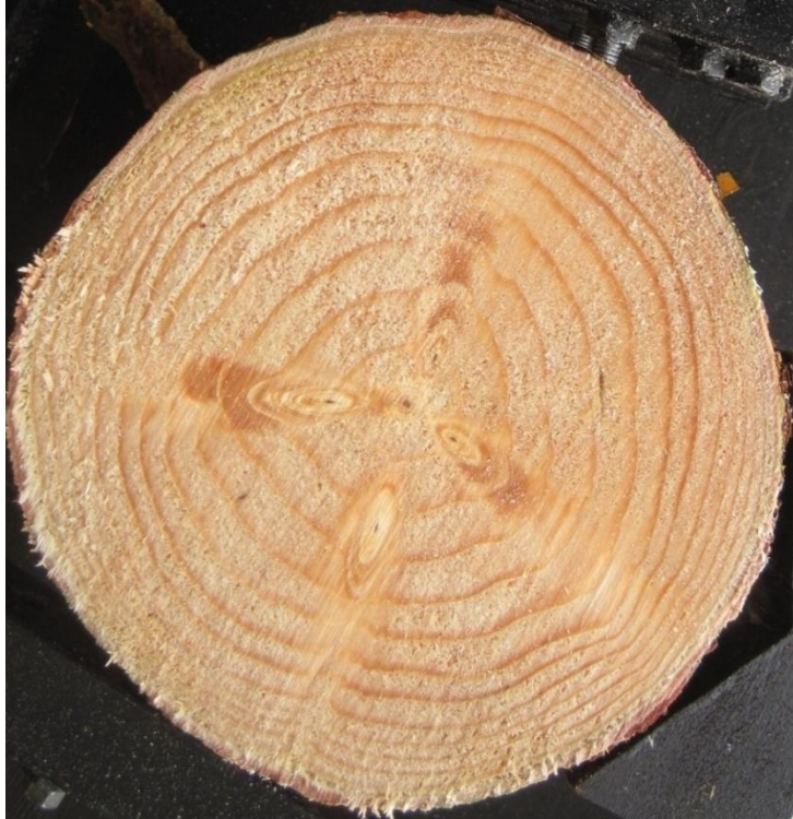
Figure 53: Resin pocket identified from photos.
