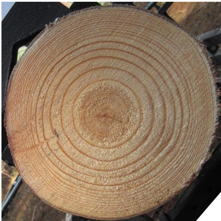
Figure 34: Resin pocket identified from photos.
