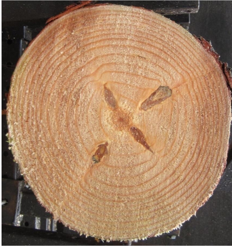
Figure 59: Resin pocket identified from photos.
