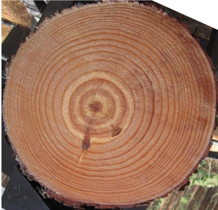
Figure 25: Resin pocket identified from photos.
