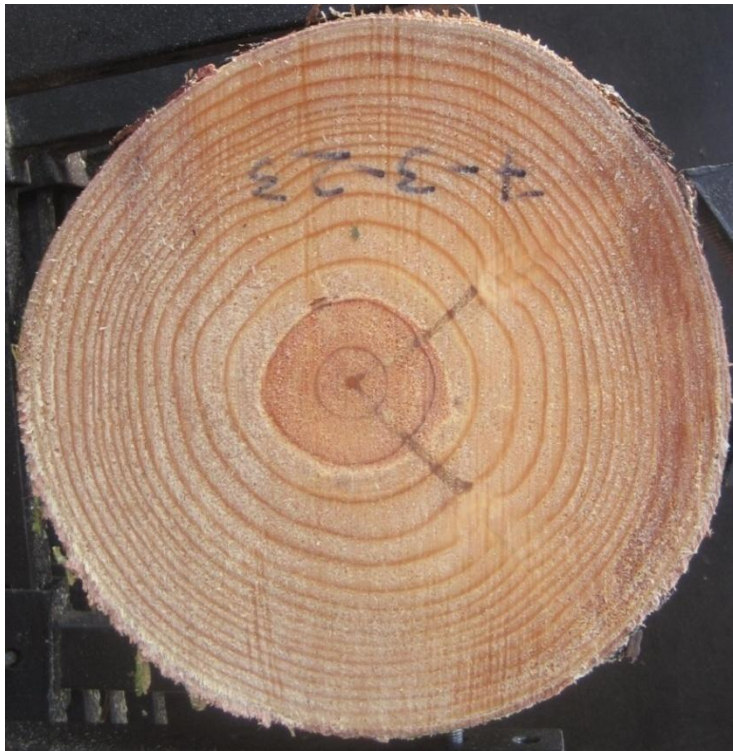
Figure 18: Resin pocket identified infield.
