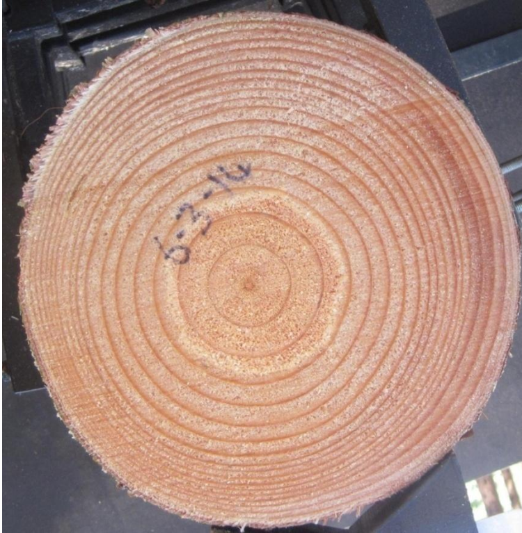
Figure 11: Resin pocket identified infield.
