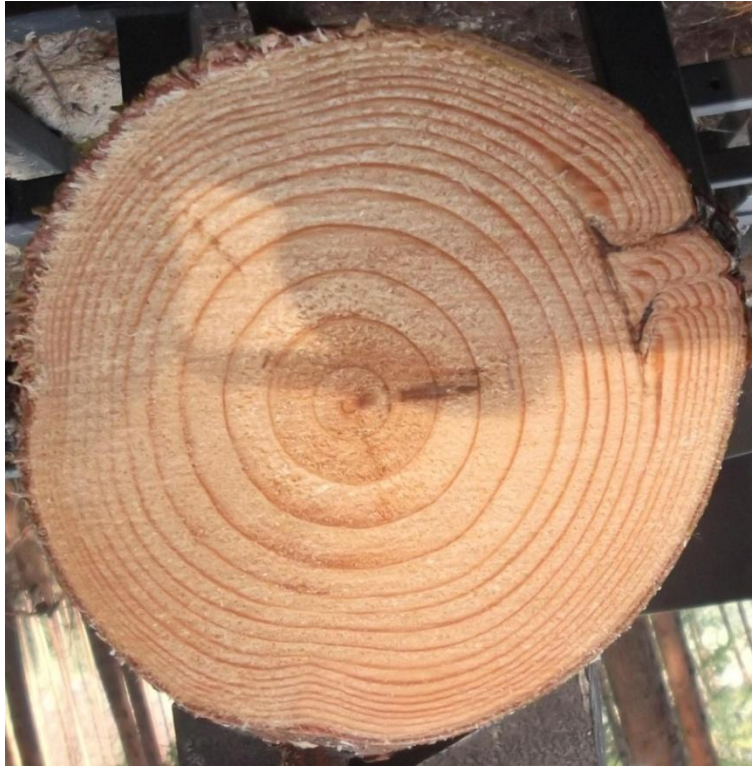
Figure 37: Resin pocket identified from photos.
