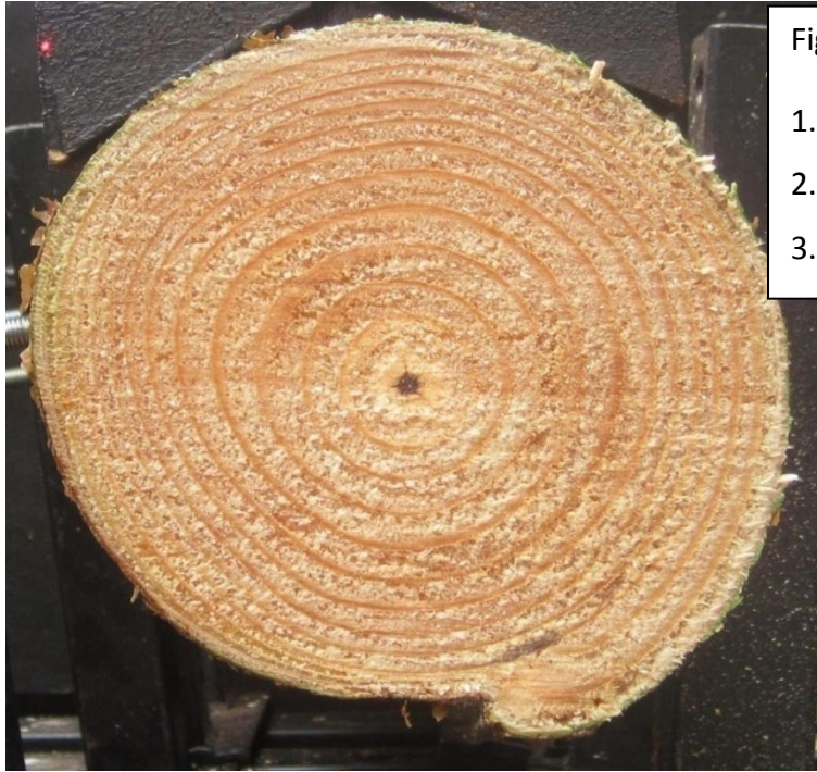
Figure 51: Resin pocket identified from photos.
