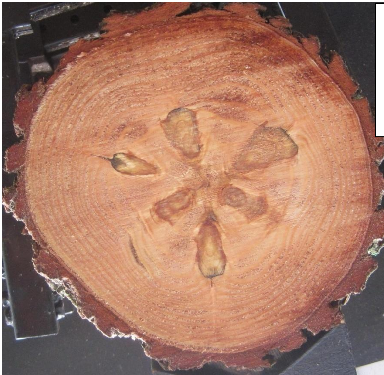
Figure 46: Resin pocket identified from photos.
