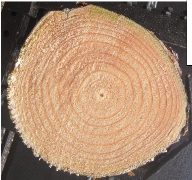
Figure 48: Resin pocket identified from photos.
