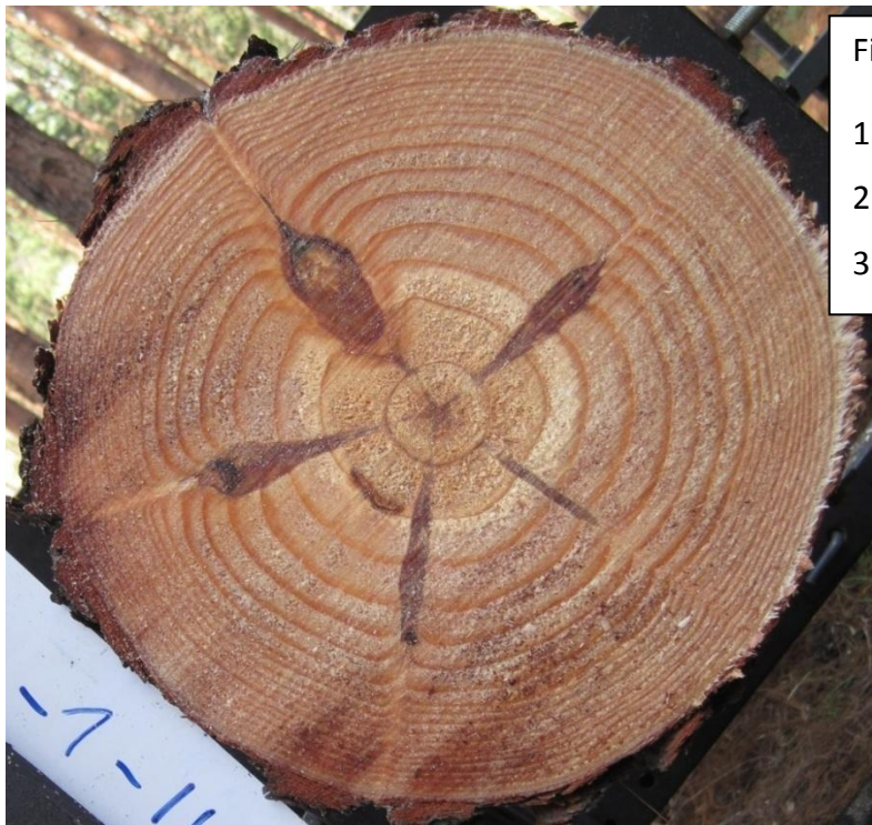
Figure 36: Resin pocket identified from photos.
