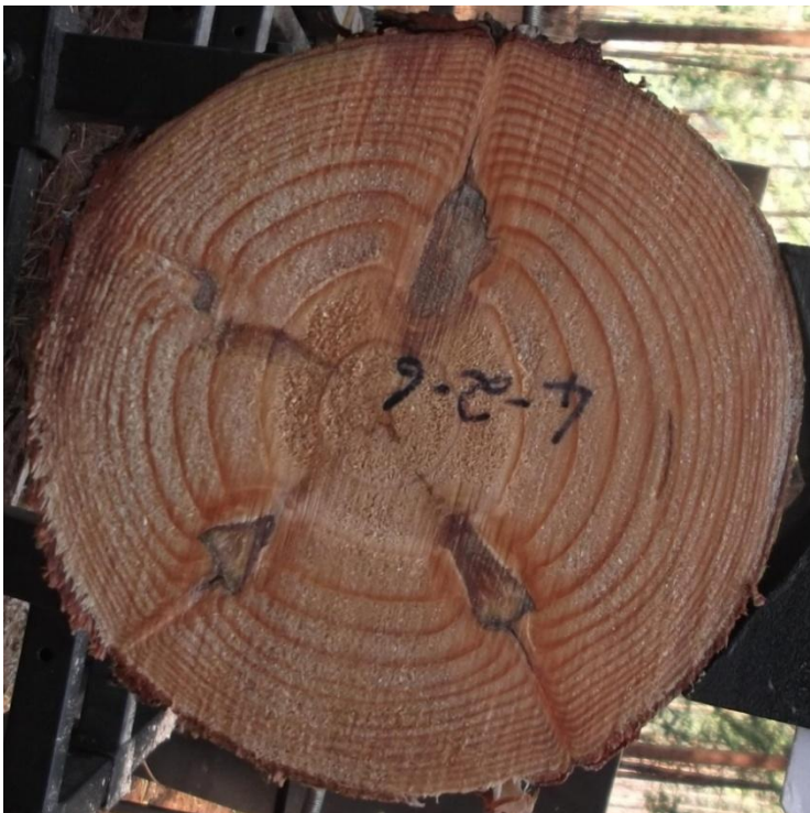
Figure 2: Resin pocket identified infield
