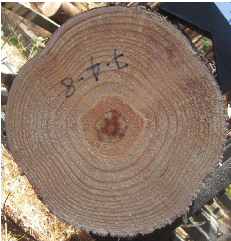
Figure 22: Resin pocket identified infield.
