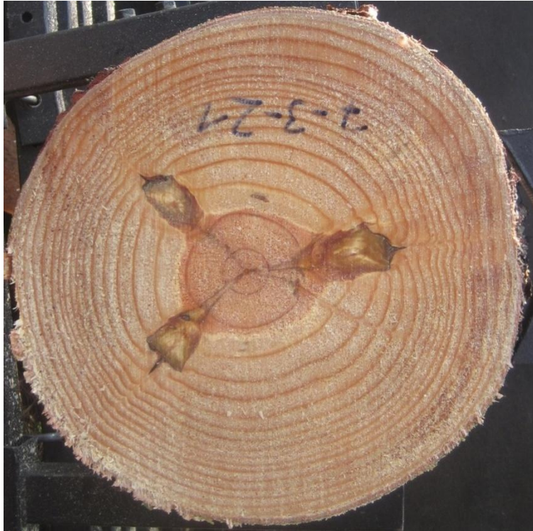
Figure 17: Resin pocket identified infield.
