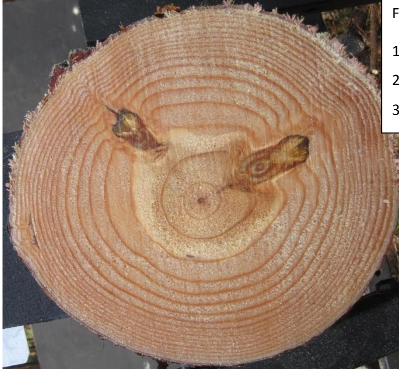
Figure 33: Resin pocket identified from photos.
