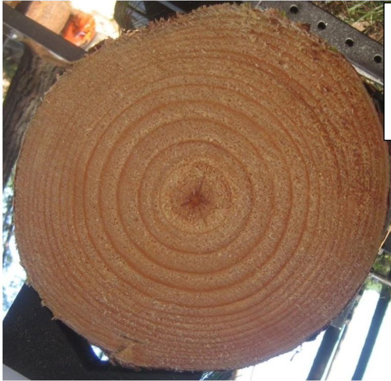
Figure 45: Resin pocket identified from photos.
