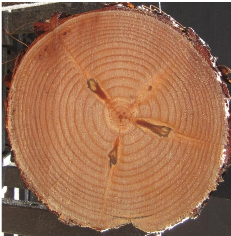
Figure 54: Resin pocket identified from photos.
