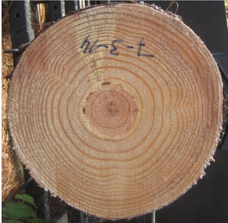
Figure 15: Resin pocket identified infield.
