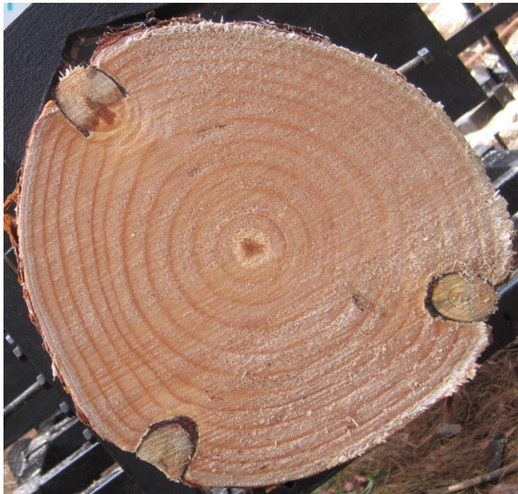
Figure 60: Resin pocket identified from photos.
