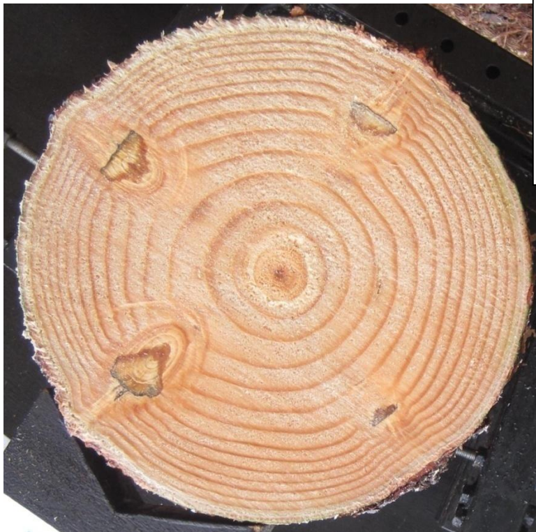
Figure 56: Resin pocket identified from photos.
