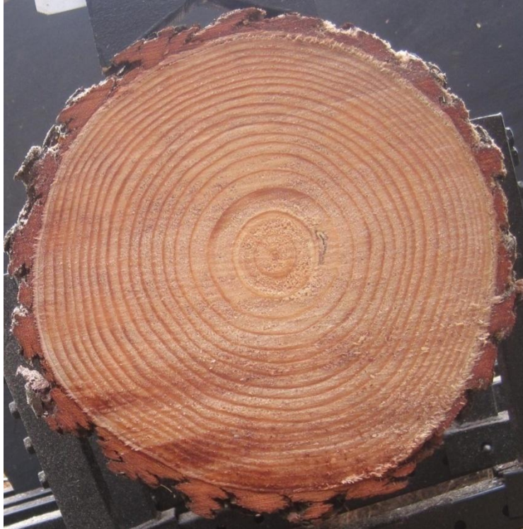
Figure 55: Resin pocket identified from photos.
