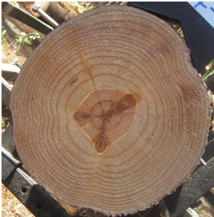
Figure 44: Resin pocket identified from photos.
