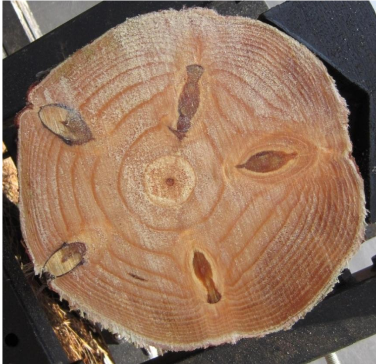
Figure 31: Resin pocket identified from photos.
