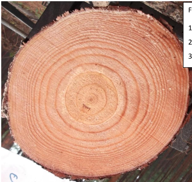
Figure 32: Resin pocket identified from photos.
