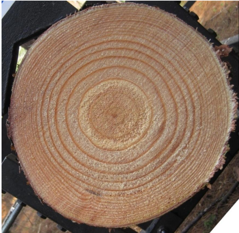
Figure 35: Resin pocket identified from photos.
