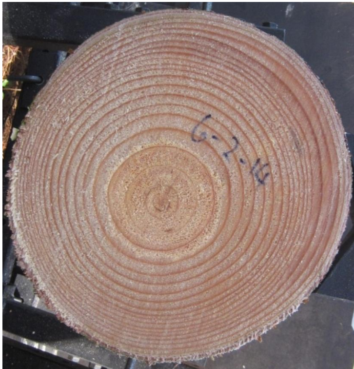
Figure 8: Resin pocket identified infield.
