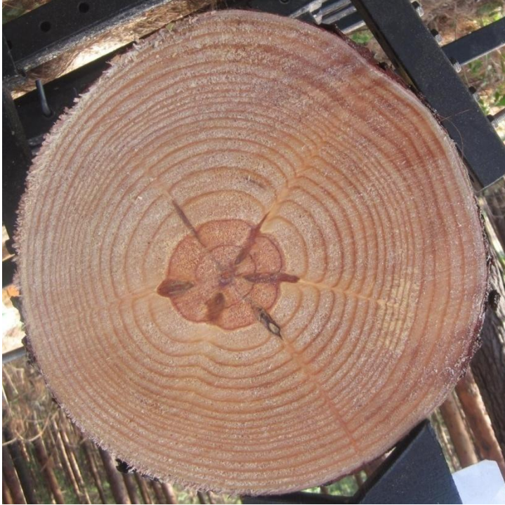
Figure 41: Resin pocket identified from photos.
