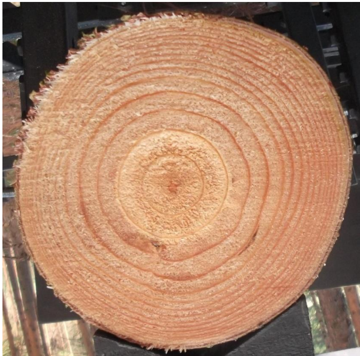
Figure 38: Resin pocket identified from photos.
