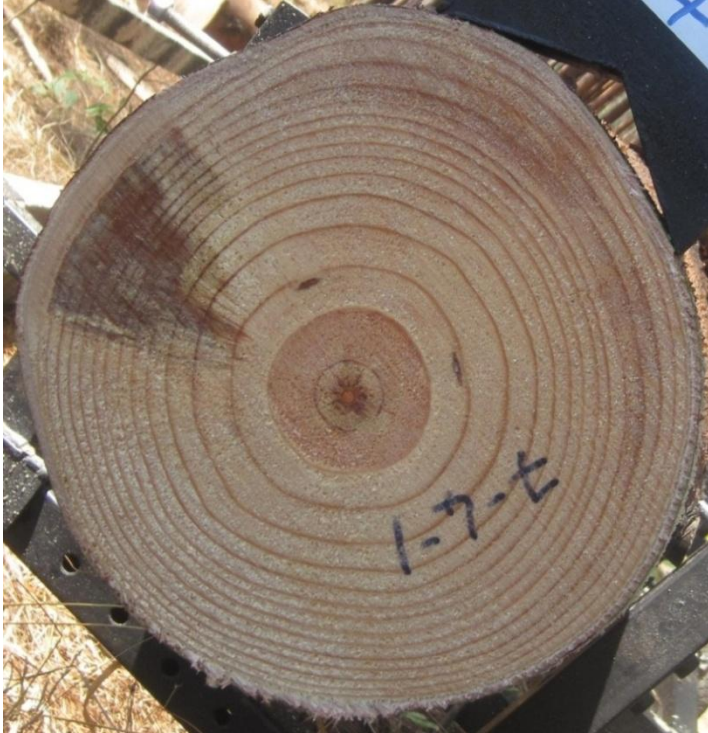
Figure 21: Resin pocket identified infield.
