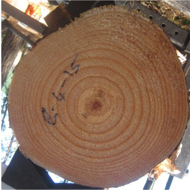
Figure 23: Resin pocket identified infield.
