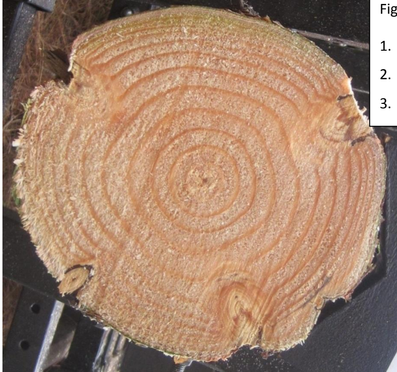
Figure 47: Resin pocket identified from photos.
