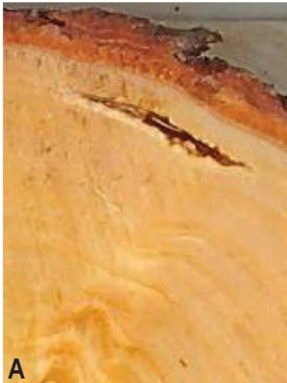
Figure 4: Type 1 resin pocket (Watt et al, 2011).
