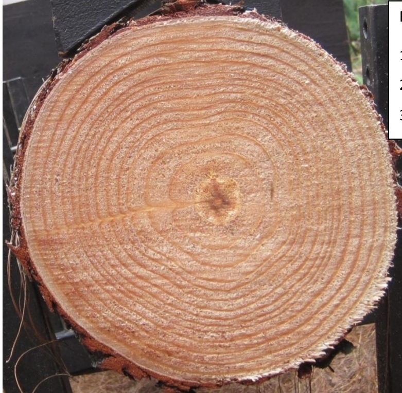
Figure 57: Resin pocket identified from photos.
