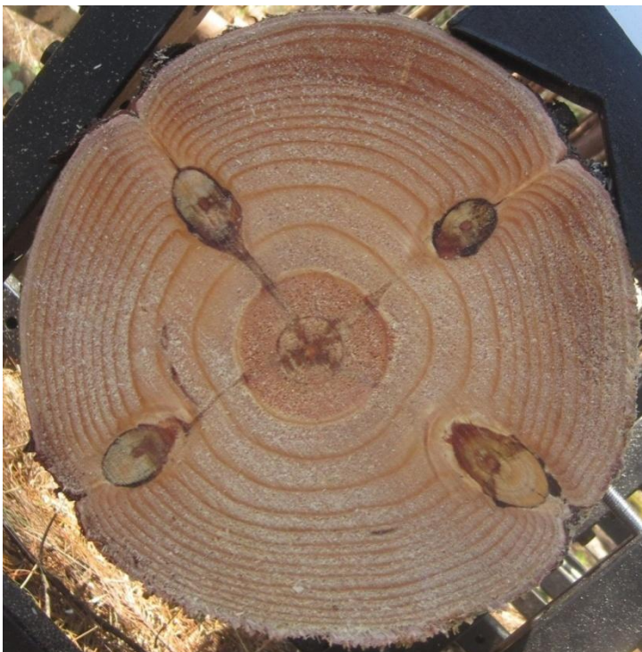
Figure 42: Resin pocket identified from photos.
