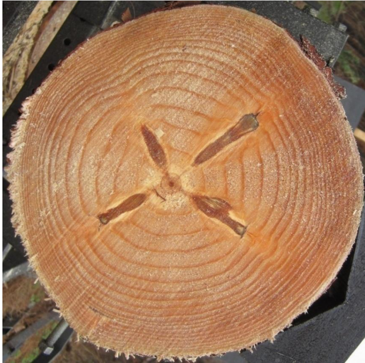
Figure 29: Resin pocket identified from photos.
