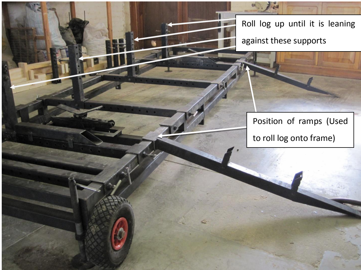
Figure 10: Figure explaining placement of ramps.
