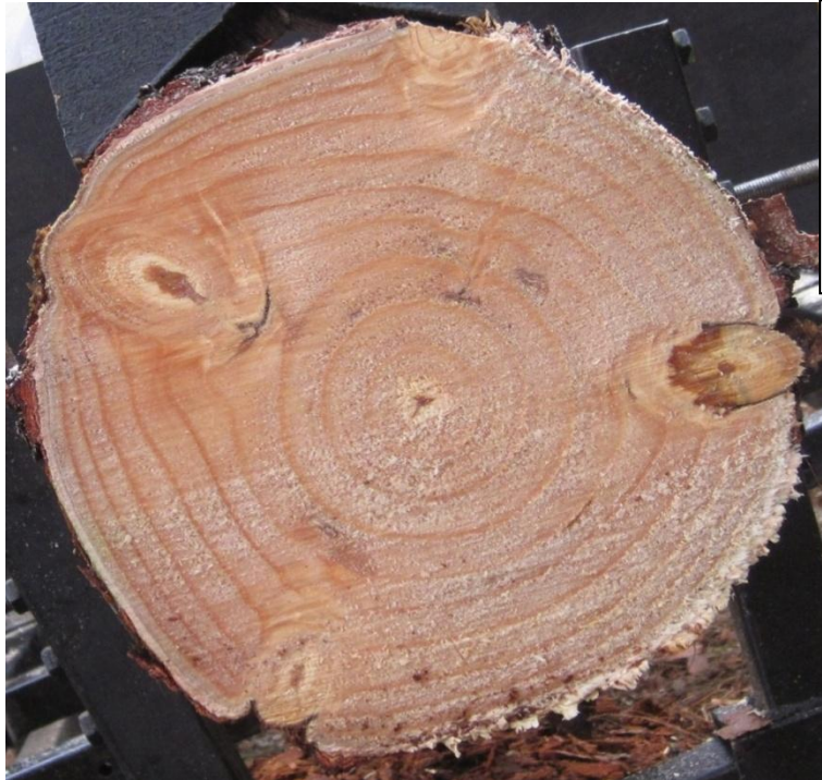
Figure 61: Resin pocket identified from photos.
