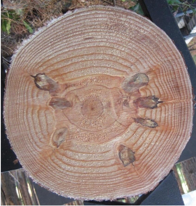
Figure 39: Resin pocket identified from photos.
