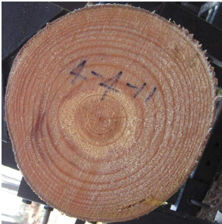
Figure 4: Resin pocket identified infield.
