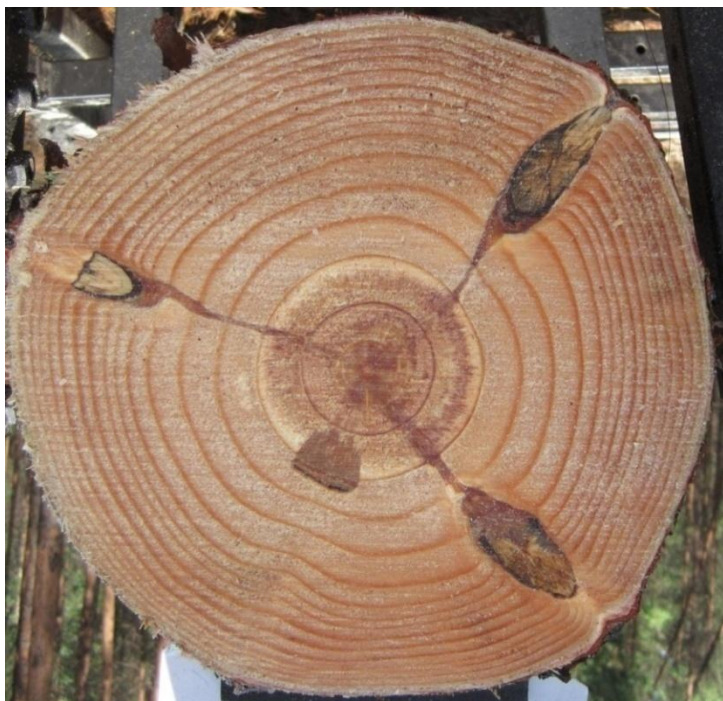
Figure 28: Resin pocket identified from photos.
