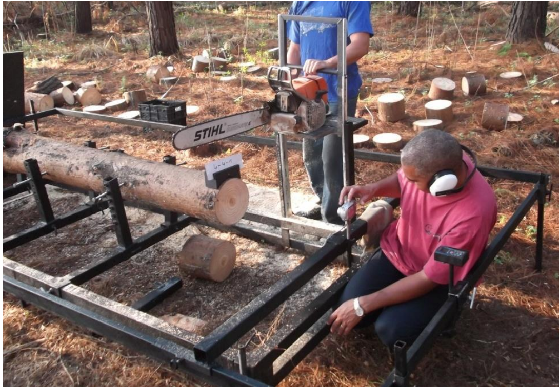
Figure 15: Image illustrating completely assembled frame infield.
