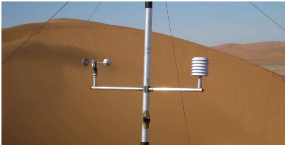
Figure 4-2: Wind speed and temperature sensor pair on wind mast
