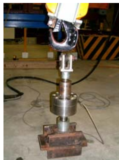
Photo 6.2: Load cell bolted to floor to simulate payload hoisting
