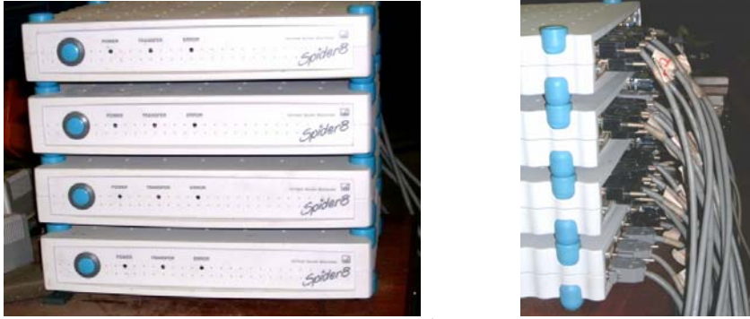
Photo B1: Spider equipment with 32 channel-input data capacity
