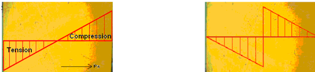
Figure C10: Typical bending stress and shear stress response in the flanges of cantilever beam
