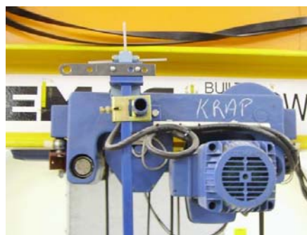
Photo 4.3: Electrical motor on crab for lateral motion
