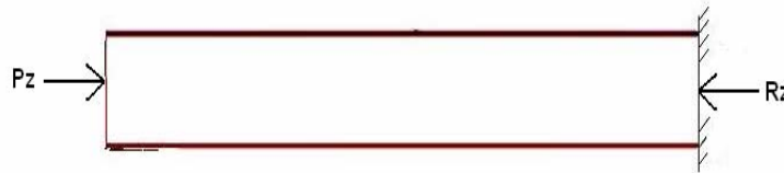
Figure C11: Elevational view of cantilever beam with applied load vector at neutral axis
