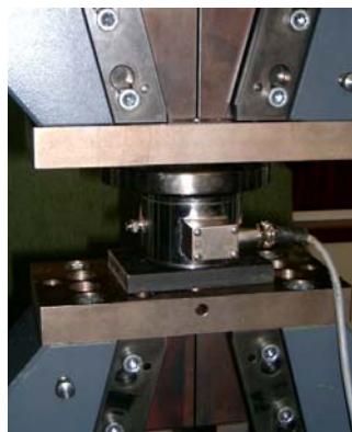
Photo 3.2: Load cell calibrated under axial load
