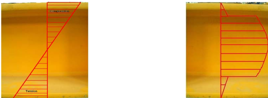
Figure C8: Typical bending stress and shear stress response in web of cantilever beam
