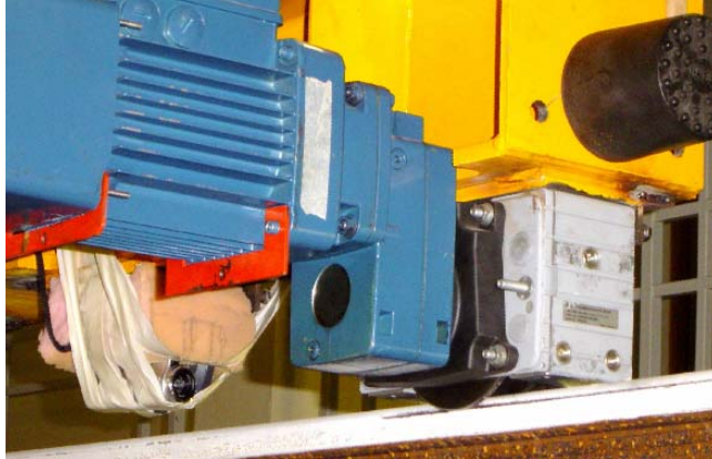
Photo F1: A digital video camera mounted close to the wheel contact surface
