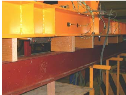
Photo A1: End carriage supported, to cancel out stress effects due to crane's own weight
