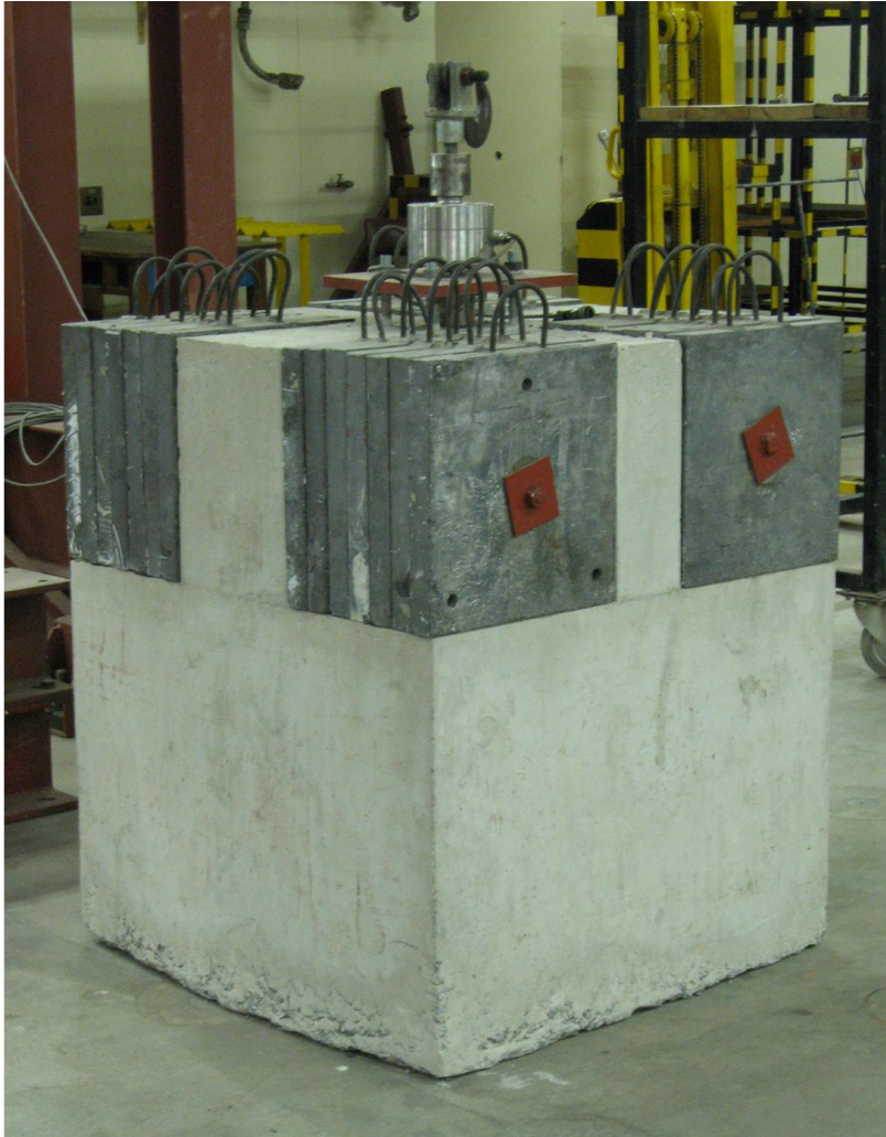
Figure 3-5: 5 ton lead and concrete payload
