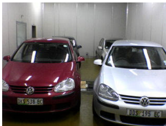
Figure 3.3: Cold-conditioning chamber used to carry out cold-start experiments
