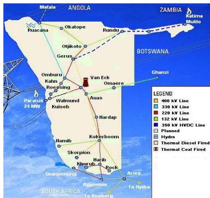
Fig. 1: Map of existing transmission lines in Namibia, also showing the planned 350 kV HVDC line (dashed blue line) [1].
