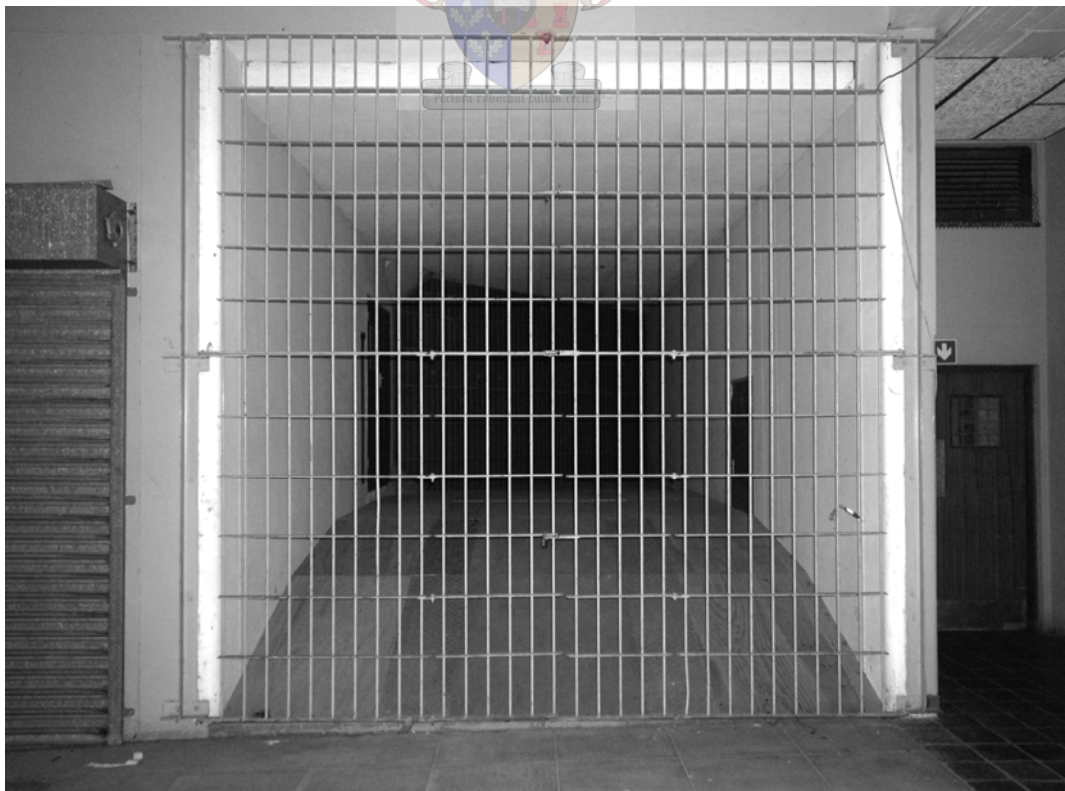
Figure 5: Wind tunnel intake section as seen from outside
