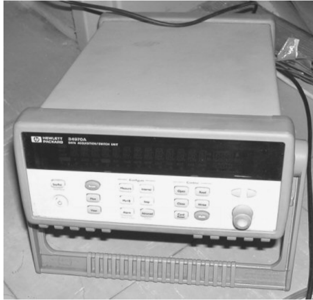
Figure 13: HP 34970A data-logger
