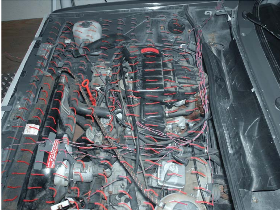
Figure 15: Visualization of airflow via Perspex bonnet
