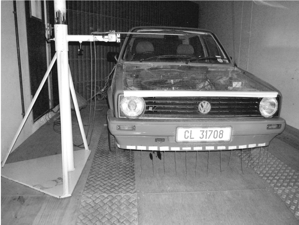
Figure 9: Vehicle parked in the tunnel with experimental apparatus in place
