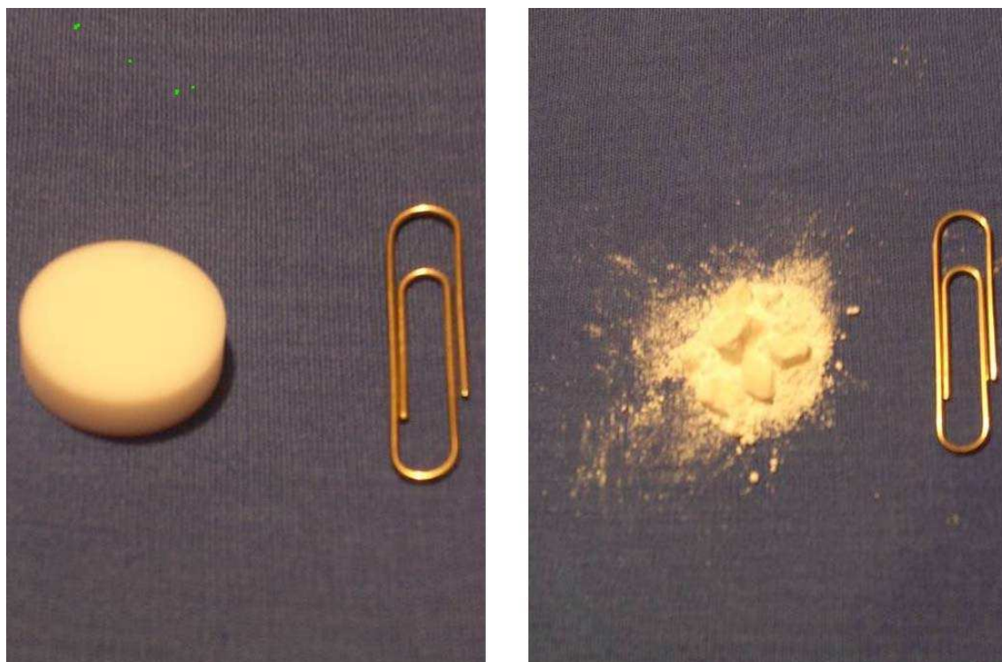
Figure 6.1: The target pellet on the left was photographed just after pressing while the photograph on the right shows the same pellet 24 hours later. This phenomenon clearly shows the effect of \text{CO}_2 absorption from the air by the \text{La}_2\text{O}_3 as explained by Bernal et. al. [57].
