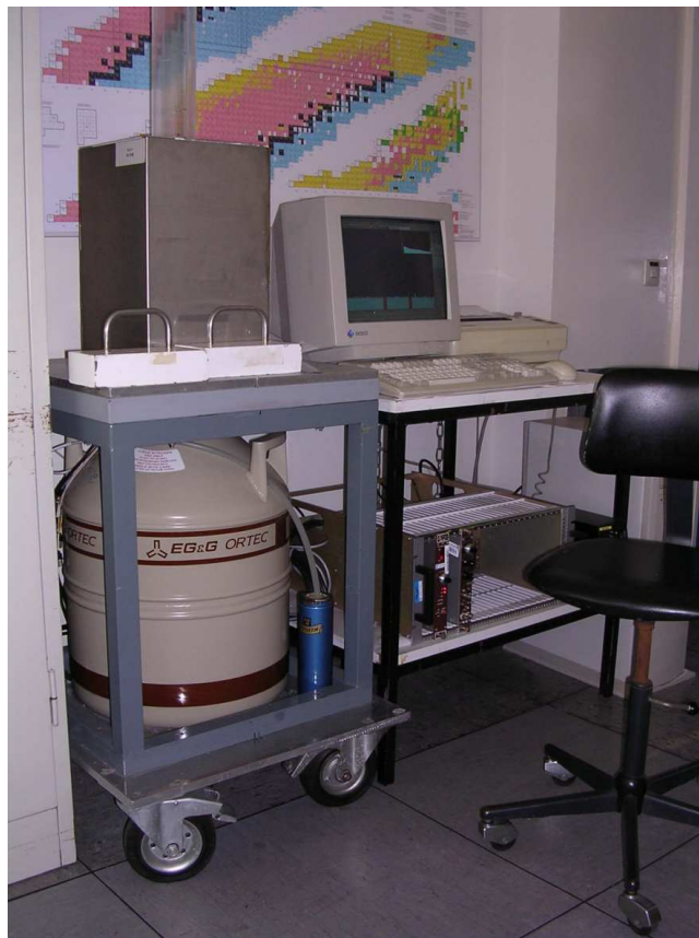
Figure 2.7: The HPGe counting facility used at the Forschungszentrum Jülich. Note the vertical geometry of the detector.
