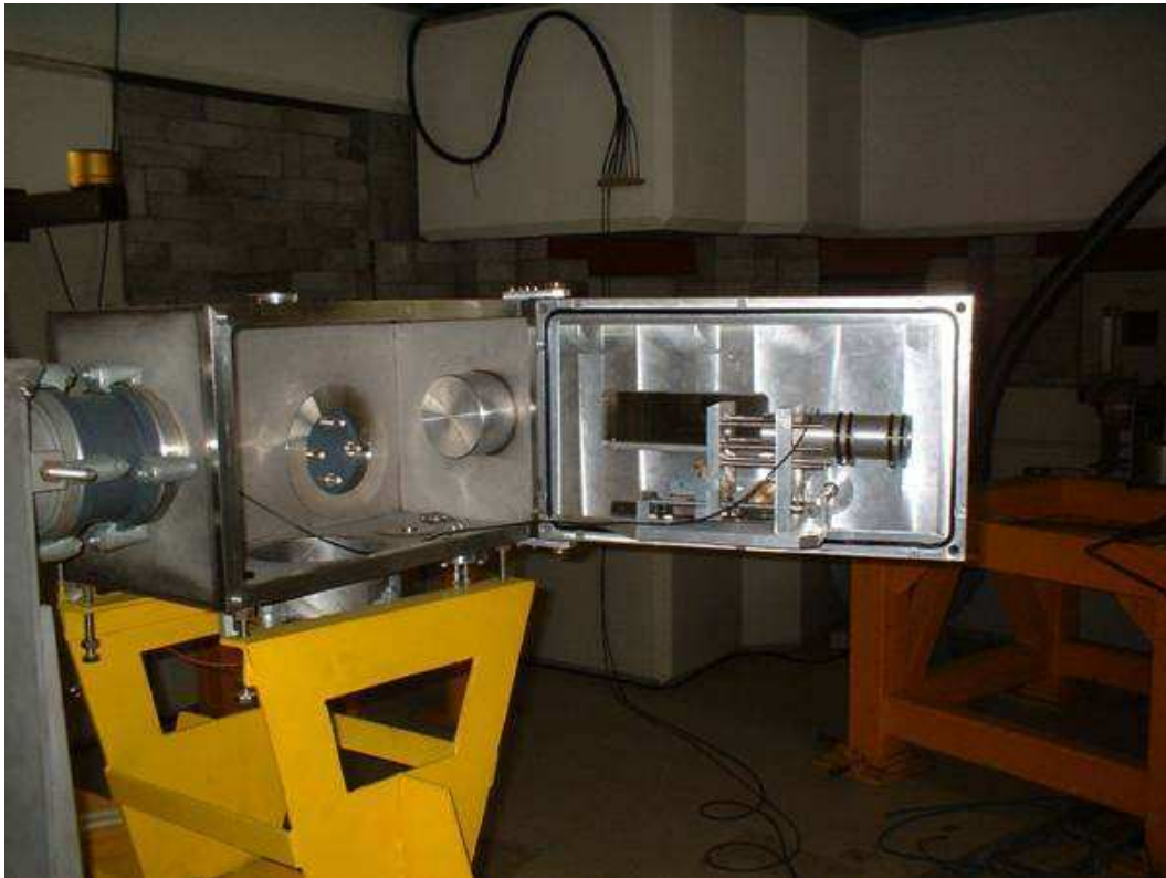
Figure 2.13: The modified RERAME irradiation chamber with the door in open position. The collimator and vice assemblies are mounted on the door. To ensure positional accuracy, the jaws of the vice move on guide rods. The beam enters the chamber from the left. (See text for further details.)
