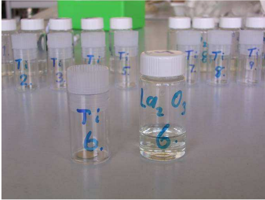
Figure 2.6: Counting sources prepared at the Forschungszentrum Jülich. The Ti monitor foils were placed in thin-walled polyethelene vials, while glass Packard vials served to contain the \text{La}_2\text{O}_3 solutions and the induced ^{139}\text{Ce} .
