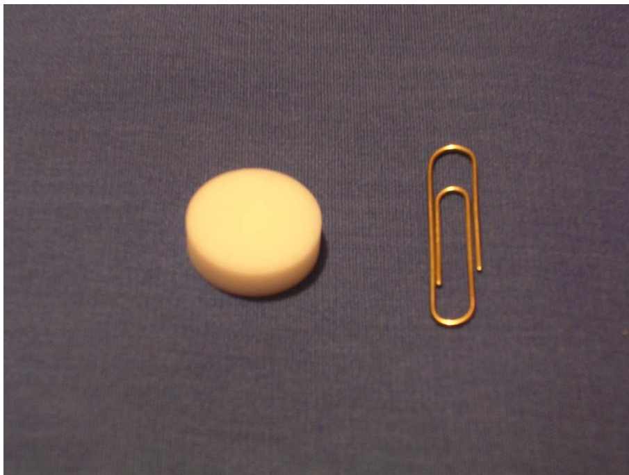
Figure 2.4: A compressed and sintered La 2 O 3 target (with a paper clip for scale).
