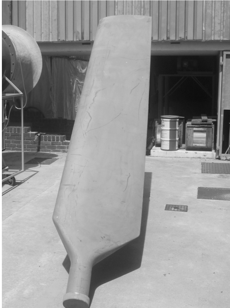
Figure B.2: Photographic image of a single fan blade of the A-fan
