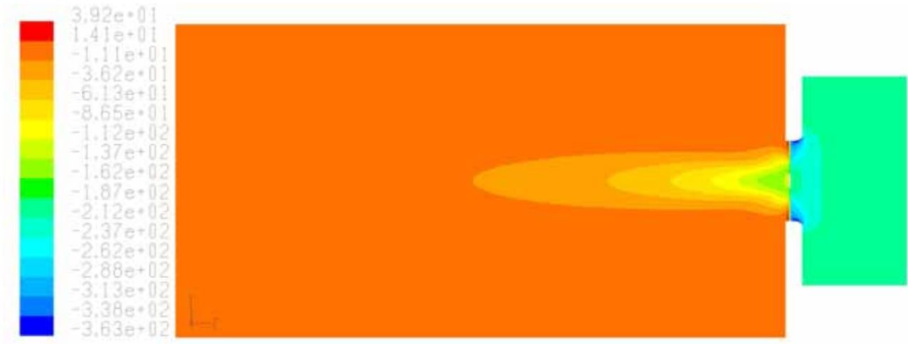
Figure 4.6: Static pressure (Pa) plot for A-fan numerical model ( d_F=9.145 m, \gamma_{pt}=16^\circ )
