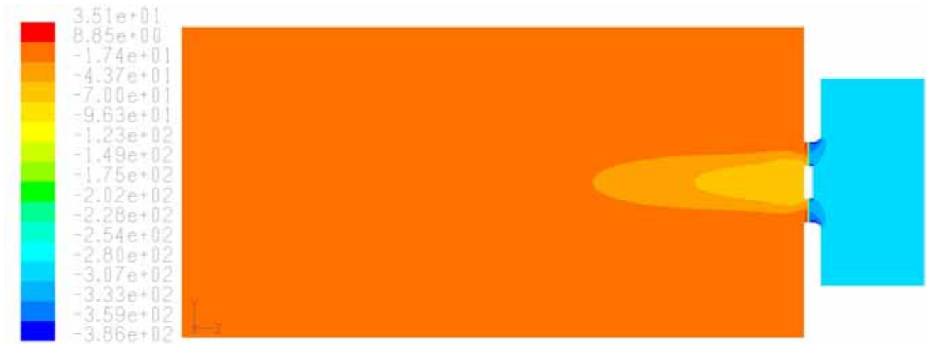
Figure 4.7: Static pressure (Pa) plot for B-fan numerical model ( d_F=1.542 m, \gamma_{cr}=31^\circ )
