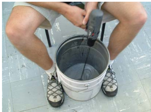
Figure 13: Mixing of the resin
