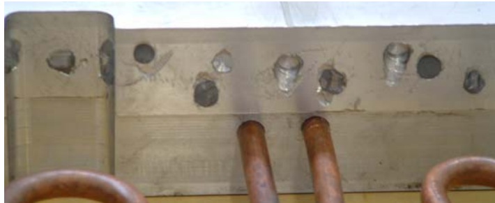
Figure 12: "Indents" inside the cavity in the cavity plate
