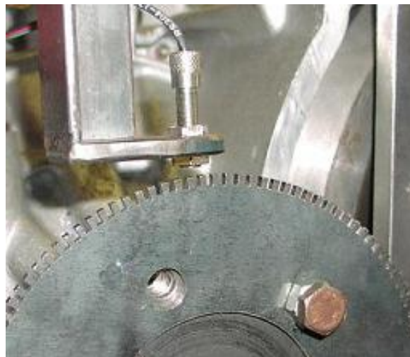
Figure 4.2.4: Digital Magnetic Pick-up Speed Measurement
