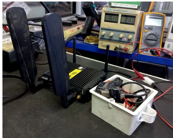
Figure 7.1: Testing with DC bench power supply
