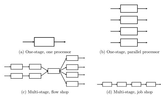
Figure 2.2: Processing structure
