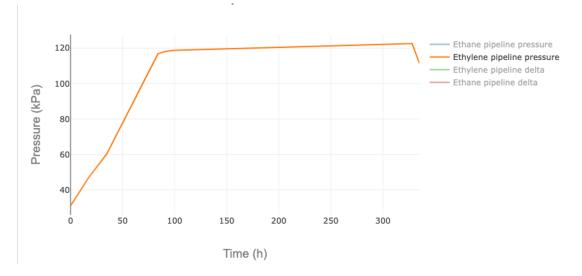
Figure 6.15: Ethylene pipeline pressure for the hourly interval downtime event
