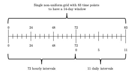
Figure 2.4: Proposed discrete-time single non-uniform grid
