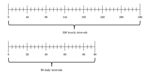
Figure 2.3: Discrete-time single uniform grids
