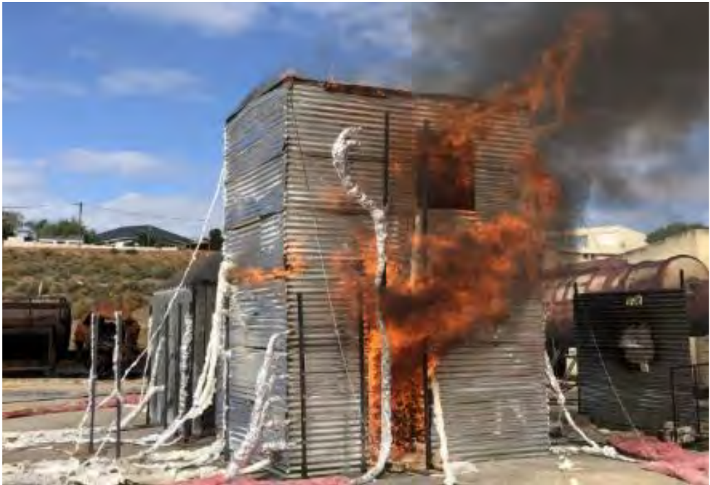
Figure 6-13: Full-scale fire test on a double storey dwelling showing the intensity of the fire
