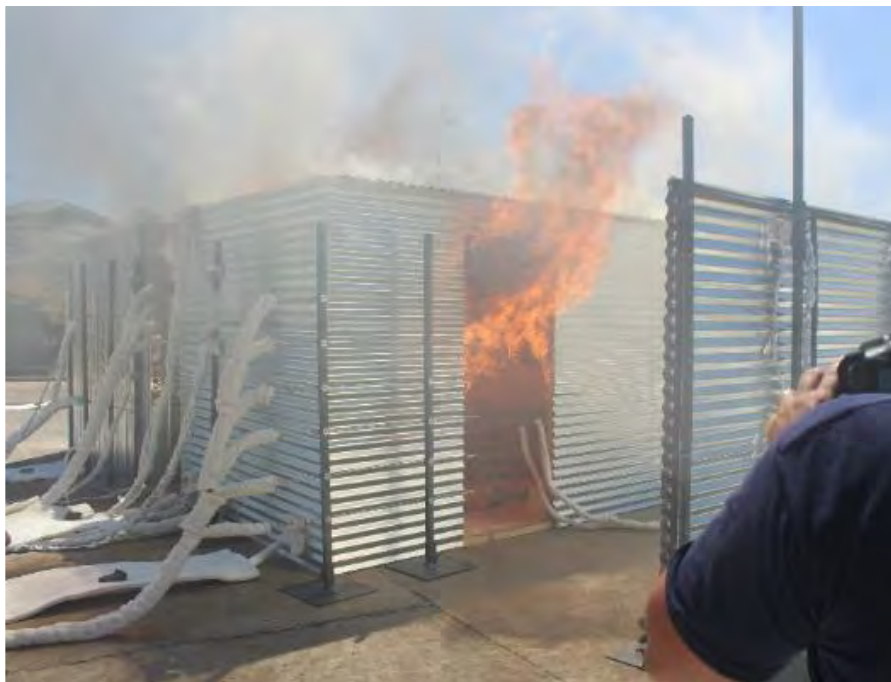
Figure 3-4: First signs of flashover during a full-scale ISD experiment
