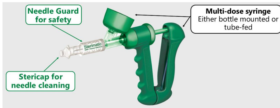
Figure 9.2 Illustration of the Sterimatic® safety needle guard system fitted with a Stericap® and mounted to a multi-dose vaccinator. The vaccinator is fitted with a 25mm metal hub needle, resulting in a 12mm injection through the needle guard and Stericap®. This system was used to immunocastrate 50 commercial Dohne Merino ram lambs, providing improved user safety from accidental needle sticks and improved hygiene through needle disinfection within the Stericap® (source: http://www.fwi.co.uk/advertisement/sterimatic-how-to-guide-for-injecting-cattle-and-sheep.htm ).
