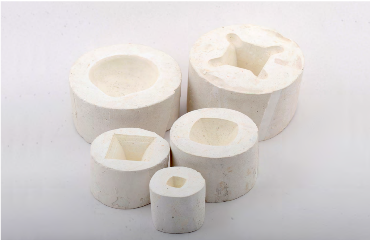
Figure 14. Ronel Jordaan, 2021: Slip cast moulds. Plaster of Paris 100 x 50 mm. Photo: Henk Kruger
