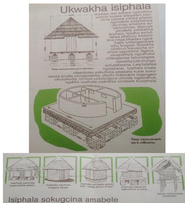
Figure 8: Pamphlet of instructions distributed to African families in the mid-1950s on how to build a granary. 211
