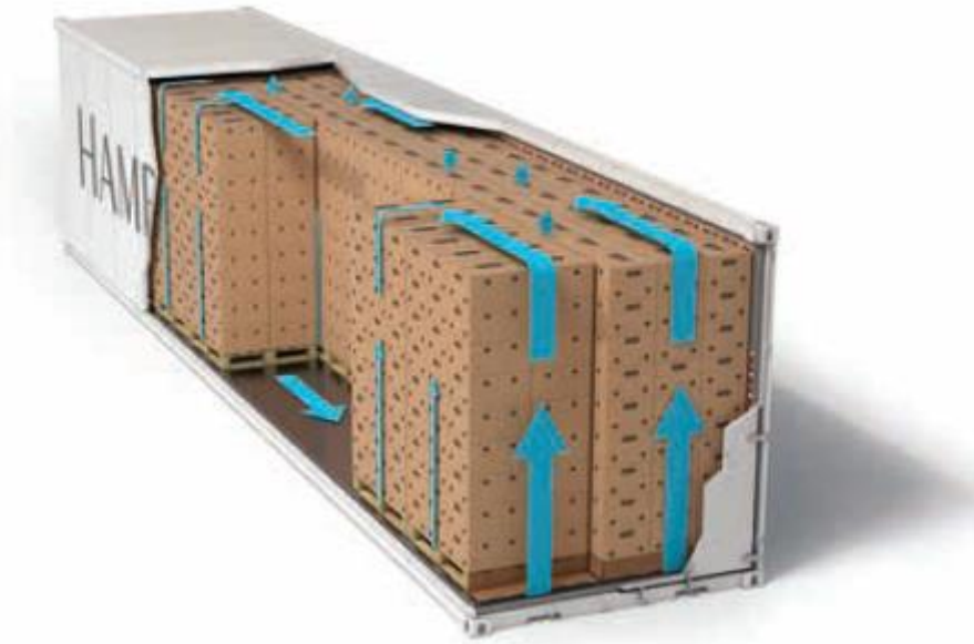
Figure 2-3: Airflow inside a container
